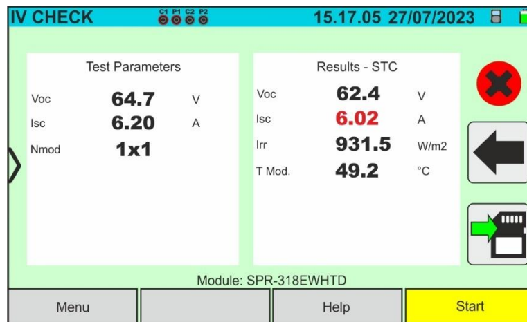
Fig. 69: Example of a negative IVCK test result - STC values
