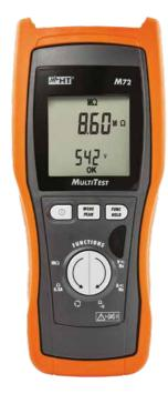
M72 is mainly dedicated to measuring **Insulation** resistance and Continuity of protective and equipotential conductors with 200mA in electric installations, typically domestic. Further to these measurements, M72 has many additional functions such as measurement of phase sequence with 1 terminal, measurement of leakage currents with optional clamp transducer and a powerful multimeter function for measuring voltage and current in true root mean square value (TRMS).
