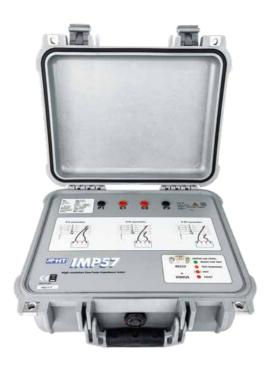
IMP57 is an optional accessory to measure Loop/Line fault loop impedance and calculating the assumed short-circuit current.
