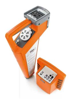
HT-5000 is a Transmitter and a Receiver which make use of the principle of propagation of the electromagnetic field on an object crossed by a signal, duly generated with different types of pairings. It is mainly used to localize metal tubes or buried cables.
