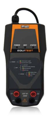
EQUITEST is designed to carry out the continuity measurement of protection and equipotential conductors with **test current >10A AC** in combination with verification instruments (MASTER unit) EASYTEST, COMBI519, COMBI521, MACROTESTG3 and GSC60 of the HT family. This accessory uses the measuring method with 4 terminals which allows the self-compensation of the resistance of the test cables and therefore their extension without the need to perform any preliminary calibration.
