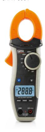
Professional clamp meter HT9012 has been designed to measure AC current up to 600A and AC/DC voltage up to 1000V to reach CAT IV 600V and CAT III 1000V in compliance with standard IEC/EN61010-1. The clamp is provided with a wide backlit display with 2000 counts and an auto power off function to preserve its battery.
