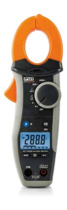
Professional clamp meter HT9014 has been designed to measure AC current up to 600A and AC/DC voltage up to 1000V TRMS to reach CAT IV 600V and CAT III 1000V in compliance with standard IEC/EN61010-1. The clamp is provided with a wide backlight display with 6000 counts and an auto power off function to preserve its battery.
