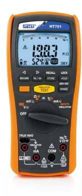
Professional **TRMS** multimeter with **10.000** measuring spots and measurement of insulation resistance with selectable test voltage among the values **50, 100, 250, 500, 1000VDC**. HT701 is capable of saving measured results in its internal **memory** and has been designed in compliance with safety standard IEC/EN61010-1 in CAT III 1000V and CAT IV 600V with double protective insulation.
