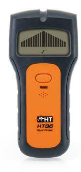
HT36 is capable of detecting the presence of wood beams and conductive items, metal items and cables with AC voltage hidden inside walls and roofs, and other common materials. The instrument gives out a sound and shows a signal on the display after identifying the border of the item, in order to easily detect its central position.
