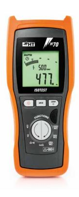
M70 is a mobile device dedicated to measuring Insulation resistance with test voltage up to 1000VDC and Continuity of protective and equipotential conductors with a current of 200 mA in domestic and industrial electric installations. Thanks to the LOCK function, insulation measurement can be carried out in a continuous
