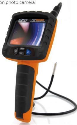
Model HTB500 is a portable digital borescope which allows carrying out inspections inside parts of objects not physically accessible (typically rotating equipment) and not visible to the naked eye. The instrument uses a waterproof external feeler with 4 LEDs with high brightness and a camera, in order to obtain a high-resolution image on the display.
