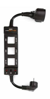
LINESPLITTER is an indispensable accessory every time you need to measure the current/power absorption or leakage current of a single-phase load supplied from socket (max 16A). This accessory separates the active conductors and the protective conductor, thus making the following measuring spots directly accessible to suitable instruments (clamp meters, clamps for measuring leakage currents, wattmetric clamps, mains analyzers):
