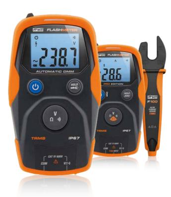
**FLASHMETER**, according to the quantity present at the input, automatically switches between voltage and resistance measurement.
