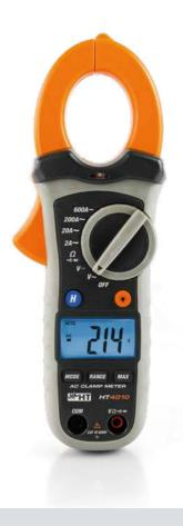
Clamp meter HT4010 can carry out measurements of AC current up to 600A and AC/DC voltage, Resistance, Continuity and Diode test. The device is provided with an internal sensor capable o detecting, through a LED turning on and a buzzer sounding, the presence of AC voltage in a spot without contact. This device complies with standard IEC/EN61010-1 in CAT III 600V and it is the ideal solution for measurements to be carried out both in domestic and in industrial environments.
