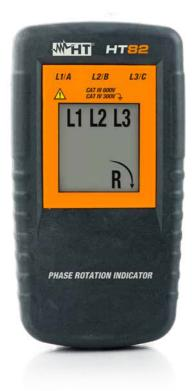
HT82 is a mobile device to display the phase sequence with 3 terminals in a generic three-phase system. The device provides an "R" indication in case of correct phase sequence or "L" indication in case of incorrect phase sequence.
