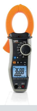
HT9021 has been designed to measure AC/DC current up to 1000A in TRMS, reaching CAT IV 600V and CAT III 1000V in compliance with safety standard IEC/EN61010-1. The clamp is provided with a display with 6000 measuring counts with backlight and bargraph to allow for a simple reading even in poorly lit environments. HT9021 also carries out measurements of voltage up to 1000V, Resistance, Frequency, Capacitance and Temperature with K-type probe.
