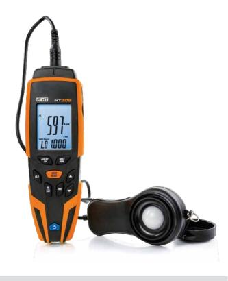
Model **HT309** is a **digital light meter** for measuring illuminance up to 400kLux through a silicon photodiode sensor. This model also allows measuring illuminance of LED sources with various colours by setting the relevant correction factors, measuring luminous intensity (expressed in Candles) and saving results in the internal memory.
