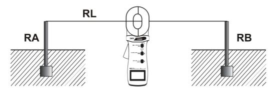
Fig. 10: Assessment of rod resistance based on two-point method
