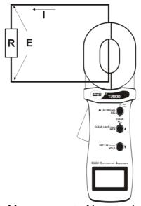
Fig. 6: Measurement of loop resistance
