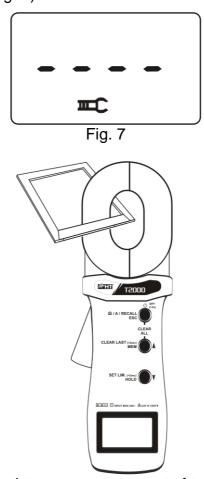
Fig. 8: Resistance measurement of test loop
