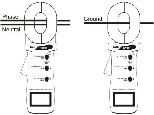
Fig. 26: Leakage current measurement
