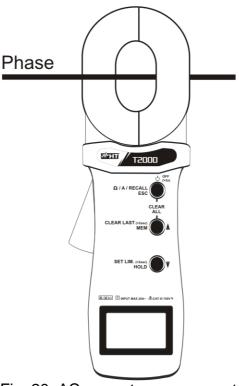
Fig. 20: AC current measurement
