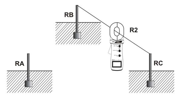
Fig. 12: Three-point method: second test R2
