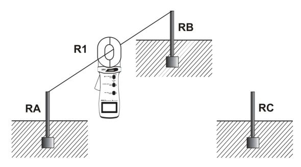
Fig. 11: Three-point method: first test R1
