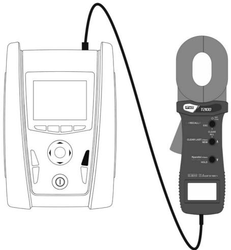
Fig. 40: Connecting T2100 to a MASTER instrument
