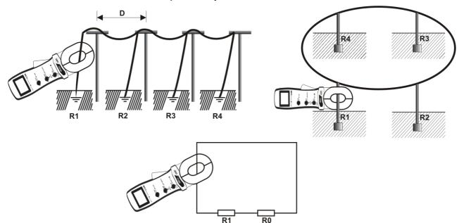
Fig. 9: Instrument's connection to a multiple-rod system
