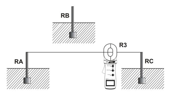
Fig. 13: Three-point method: third test R3
