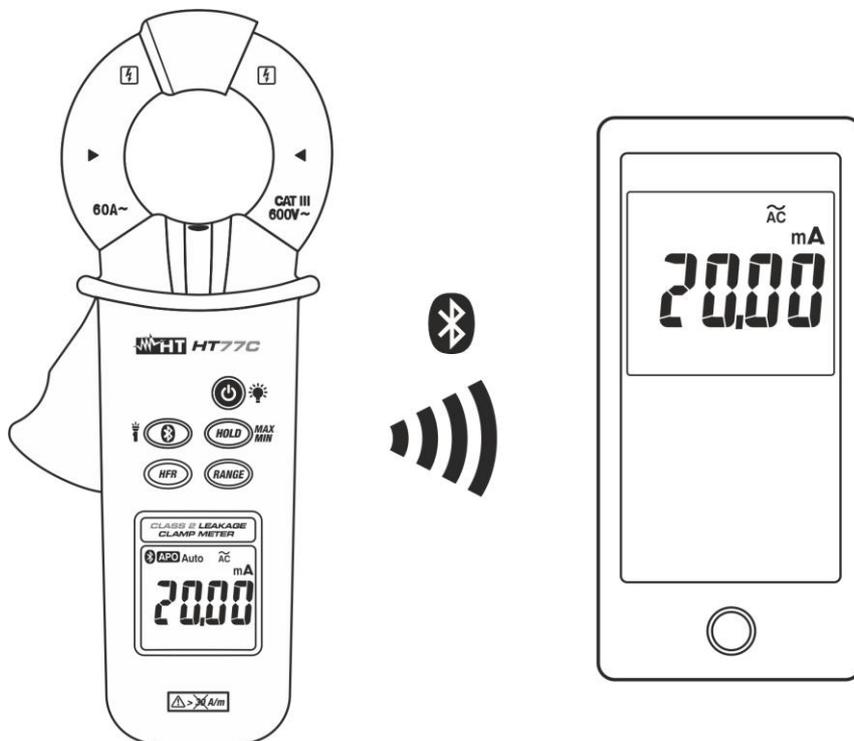
Fig. 8: Connection of instrument to a mobile device
