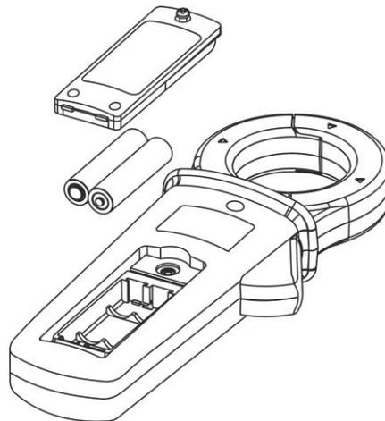
Fig. 9: Batteries replacement
