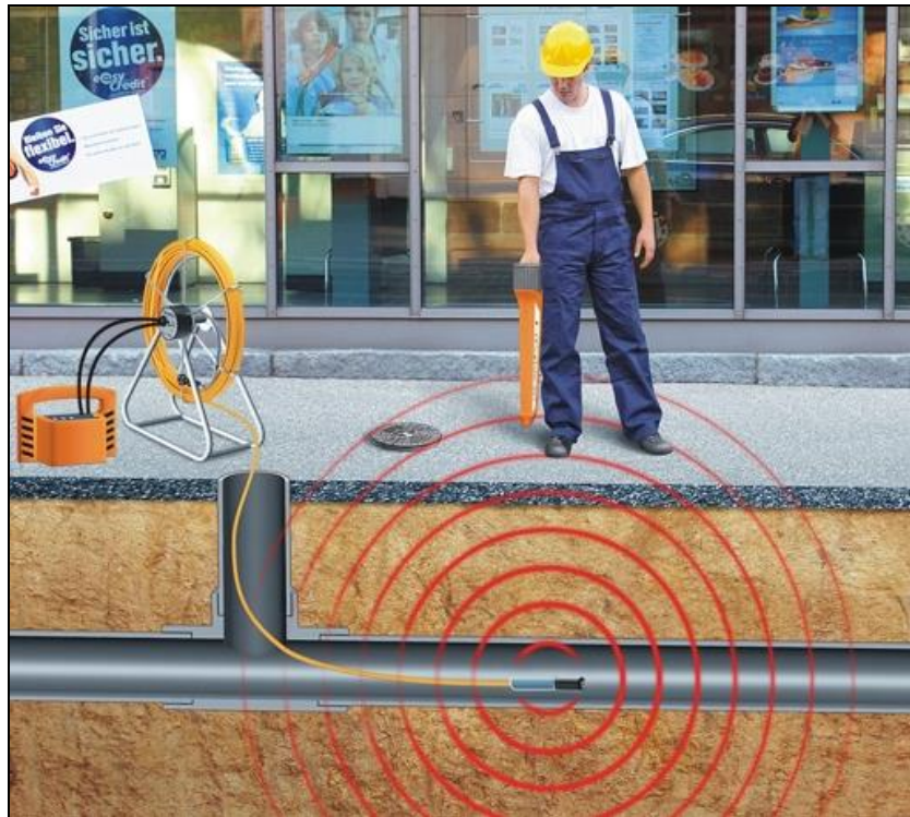
Fig. 9: Signal coupling in non-metallic pipes
