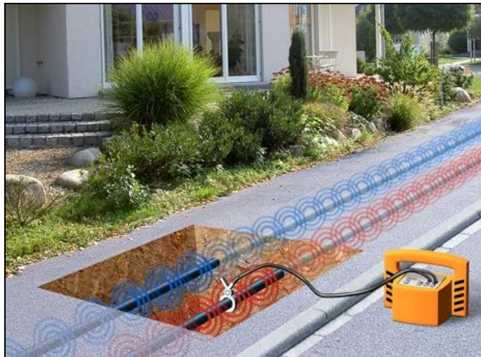
Fig. 6: Coupling via transmitter clamp
