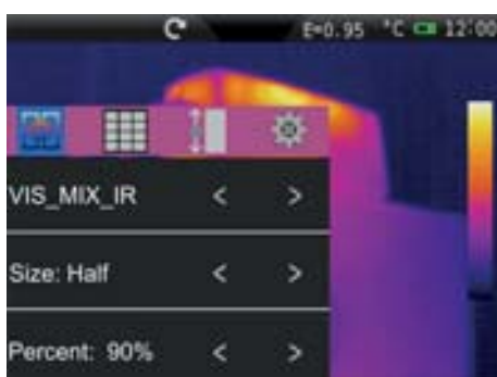
Fig. 46: Setting and displaying the VIS_MIX_IR image
