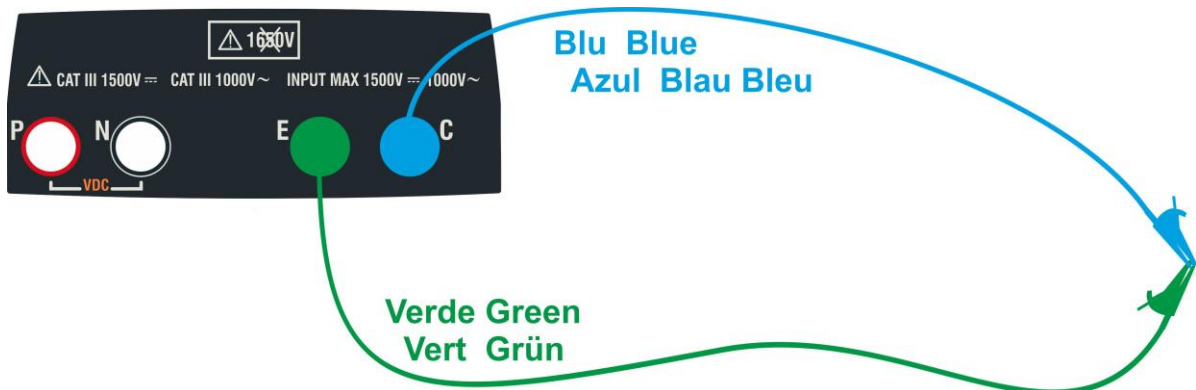
Fig. 4: Compensation of the measuring cables resistance
