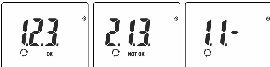
Fig. 14: Results of phase sequence and phase concordance test
