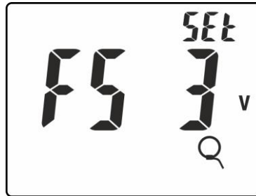
Fig. 5: Setting the full scale for flexible clamp transducer
