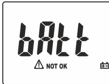
Fig. 43: Screen with low battery indication
