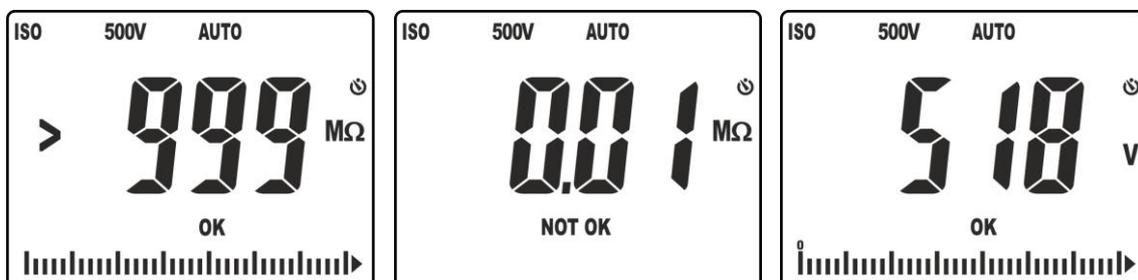
Fig. 18: Results of insulation measurement in AUTO mode
