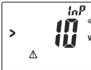
Fig. 17: Presence of voltage on the input terminals
