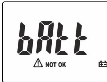
Fig. 43: Screen with low battery indication
