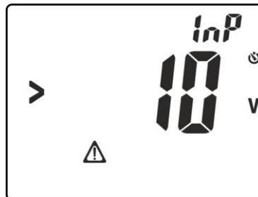
Fig. 27: Presence of voltage on the input terminals
