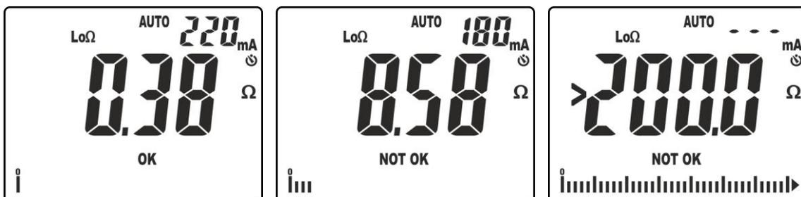
Fig. 28: Results of continuity test in AUTO mode
