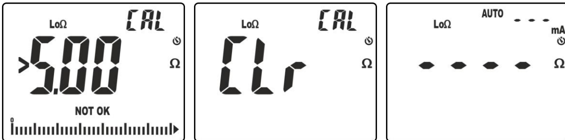
Fig. 34: Results of zeroing not correctly performed
