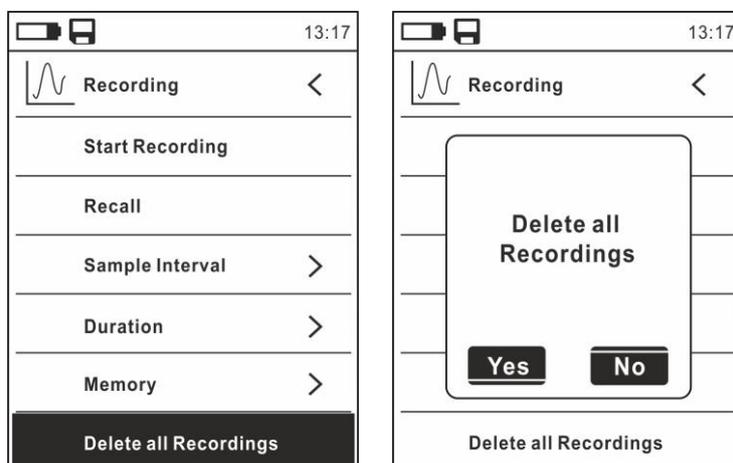
Fig. 38: Data logger function – Deleting all recordings
