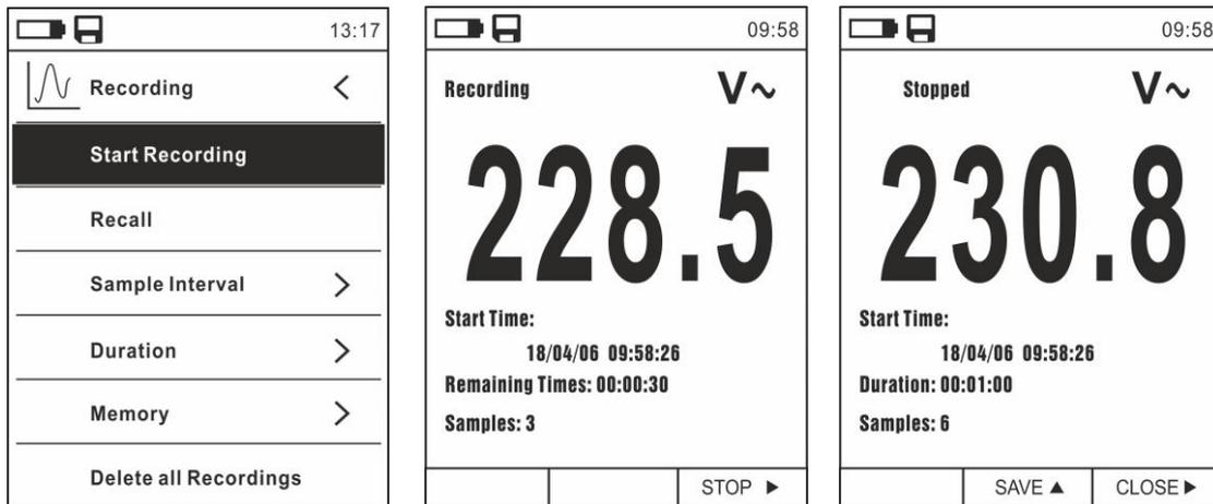
Fig. 33: Data logger function – Starting and stopping recording
