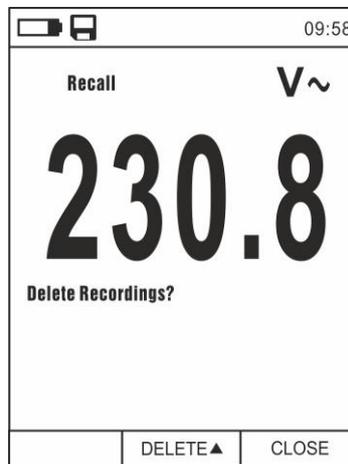
Fig. 36: Data logger function – Deleting recorded data
