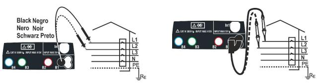
Fig. 24: Phase sequence check of 1T phases with terminal and remote lead
