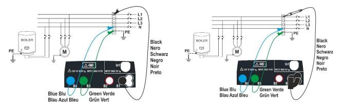
Fig. 10: Insulation test between L-PE and N-PE by means of single cables and remote lead
