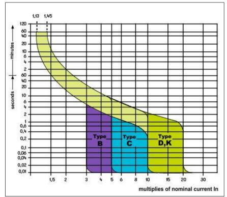
Fig. 46: Example of curves relative to magnetothermal (MCB) protection
