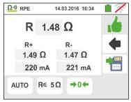
The symbol indicates the positive result of the measurement.
