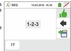
At the end of the test, if the two detected voltages are in phase (phase concordance between two distinct three-phase systems), the instrument displays a screen like the one to the side (result "1-1-").
