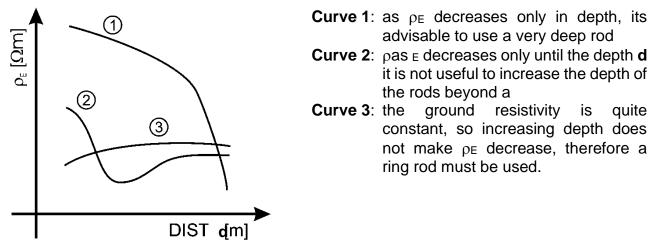
Fig. 50: Ground resistivity measurement
