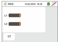
Move the slide bar reference in the position "1T" for the selection of the test with 1 terminal or in the position "2T" for the selection of the test with 2 terminals.
