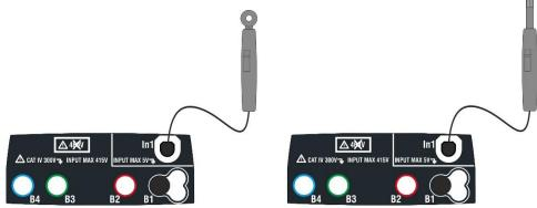
Fig. 33: Measurement of environmental parameters through external probes
