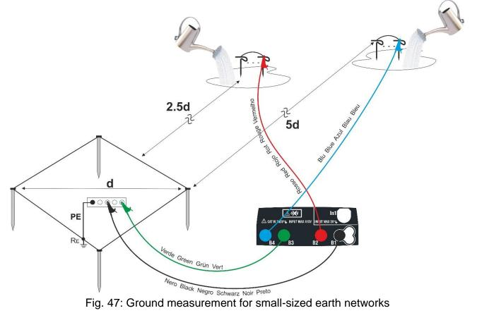
If needed, use multiple probes in parallel and wet the surrounding ground (see Fig. 47) if the instrument is not able to supply the current required to perform the test due to a high resistance of the ground.
