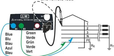
Fig. 23: P-PE measurement for IT systems by means of single cables and remote lead EN - 39
