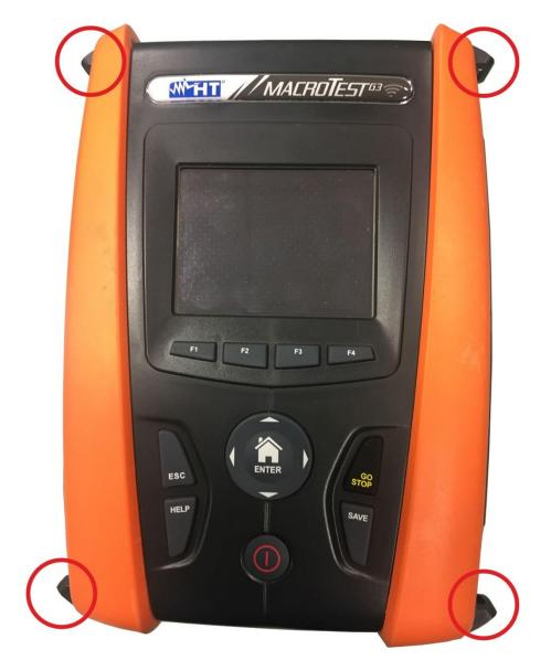
Fig. 42: Instrument with fitted half-shells and hooks
