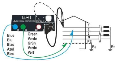
Fig. 21: P-P measurement for 400V+N+PE three-phase systems
