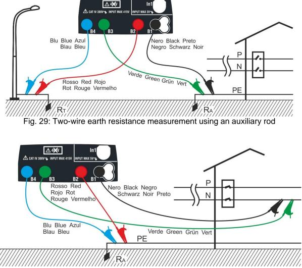
Fig. 30: Two-wire earth resistance measurement from the panel board
