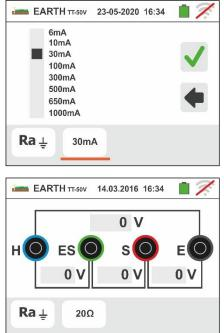
Touch the  $\bowtie$  icon to zero the value in the " $\Omega$ " field and use the virtual keyboard to set the value of limit earth resistance between  $\mathbf{1}\Omega$  and  $\mathbf{999}\Omega$ . Confirm the choice by going back to the initial measurement screen.
