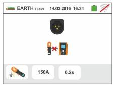
2. Connect the clamp T2100 by inserting the connector into input **In1** of the instrument. Turn the clamp on and put it in "RS232" mode (see the user manual of the clamp). The **232**<sup>5</sup>
