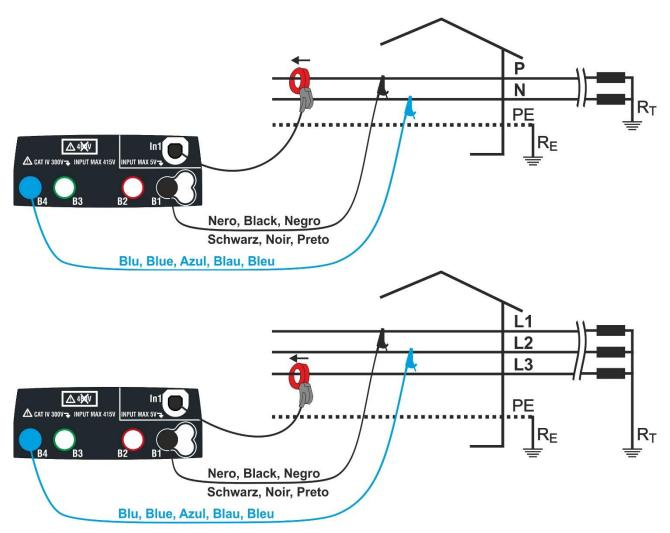
Fig. 37: Connection for measurement on Single phase installations
