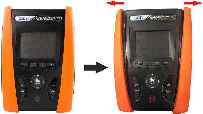
Fig. 40: Remove lateral half-shells
