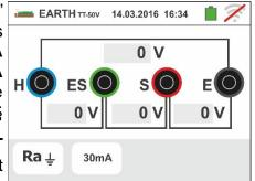
Touch the first icon in the lower left corner to set the measuring mode. The following screen appears on the display:
