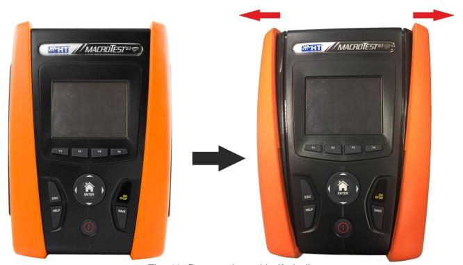
Fig. 40: Remove lateral half-shells
