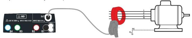
Fig. 26: Indirect measurement of leakage current in three-phase systems
