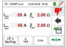
9. If the electrical Noise between N and PE conductors is so high that it could compromise the result accuracy, the symbol is displayed. It's recommended to switch off all the electrical loads and re-attempt the measurement
