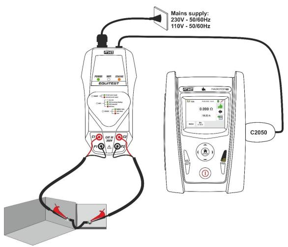
Fig. 36: Continuity test by means of EQUITEST accessory
