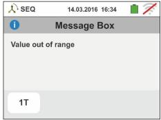
3. If the instrument detects an input voltage frequency exceeding the allowed full scale, it will display a screen like the one to the side.
