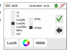
In case of LED/colored sources it is necessary to set the correspondent color temperature value (expressed in K) in the range: 2500K ÷ 6500K in order to have a correct measurement result
