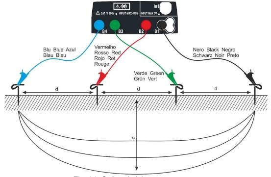
Fig. 31: Soil resistivity measurement EN - 74
