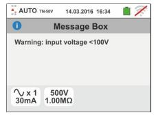
If the instrument detects the absence of the signal to terminal B1 (phase conductor), it provides the warning screen shown to the side and blocks the execution of the tests
