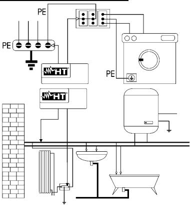
Connect one of the test leads to the protective conductor of the socket and the other to the equalizing potential node of the earth installation.
