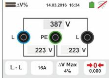
Move the second slide bar reference and select the type of measurement between the options: L-L (Phase-Phase measurement) or L-N (Phase-Neutral measurement).
