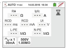
8. In case of **positive** result of the three test sequentially performed as **NoTrip**<sup>‡</sup> (see § 13.8), **RCDX1** (see § 13.4) and **MΩ L/N-PE** the screen to the side is displayed by the instrument
