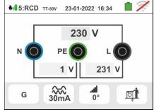
58 Move the third slide bar reference by selecting the desired rated current of the differential switch between the options: **6,10, 30, 100, 300, 500, 650mA**
