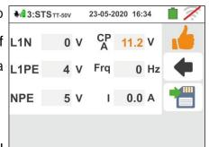
23 If the test fails, the screen like the one on the side is shown on the display. The incorrect value of the parameter is shown in red and the symbol indicates the non-ok result of the measurement
