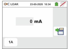
2. Touch the icon to zero the value in the In field and use the virtual keyboard to set the full-scale value of the clamp used ((values of 1A, 100A, 1000A for the HT96U clamp).
