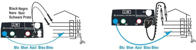
Fig. 25: Phase sequence check of 2T phases with terminal and remote lead
