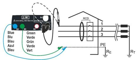
Fig. 16: Connection for a 400V + PE (no N) system with single cables and remote lead
