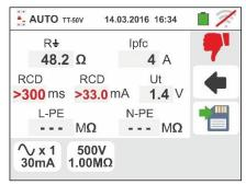
13 In case of **negative** result of the  $M\Omega$  **L-PE**, the auto test is automatically blocked, the symbol is shown and the screen to the side is displayed. Note red value (lower than minimum set trhreshold) of the L-PE insulation resistance
