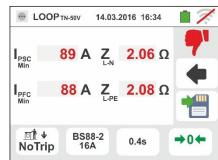
9. If the electrical Noise between N and PE conductors is so high that it could compromise the result accuracy, the symbol is displayed. It's recommended to switch off all the electrical loads and re-attempt the measurement
