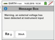
When starting a measurement, the instrument checks the continuity of measuring cables. If the <u>voltmetric</u> circuit (red cable S and green cable ES) is interrupted or its resistance value is too high, the instrument displays a screen similar to the one on the side.
