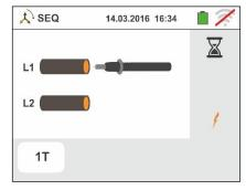
7. The symbol for the tip on phase L2 and the hourglass indicating the status of pending recognition of a voltage higher than the maximum allowed.
