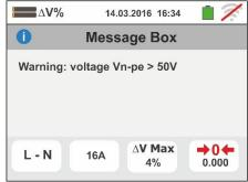
10 If during the measurement the instruments detects an end of line impedance value lower than the initial line impedance value it does not carry out the test and a screen similar to the one reported to the side is displayed. Check the status of the main line being tested
