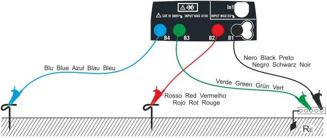
Fig. 28: Three-wire earth resistance measurement
