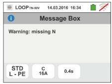
If the instrument detects the absence of the signal to terminal B3 (PE conductor), it provides the warning screen shown to the side and blocks the execution of the tests.
