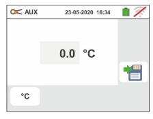
2. Move the left slide bar reference to select the type of measurement among the options: °C (temperature in Celsius degrees), °F (temperature in Fahrenheit degrees), Lux(20) (illuminance with 20Lux capacity), Lux(2k) (illuminance with 2kLux capacity), Lux(20k) (illuminance with 20kLux capacity) ,%RH (relative humidity), mV (measurement of DC voltage up to 1V). Move the right slide bar reference to select the model of optional probe for illuminance measurement between the options:
