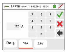
Touch the icon to zero the value in the "s" field and use the virtual keyboard to set the value of the time for fault elimination t (declared by the Energy distribution board) between **0.04s** and **10s**.
