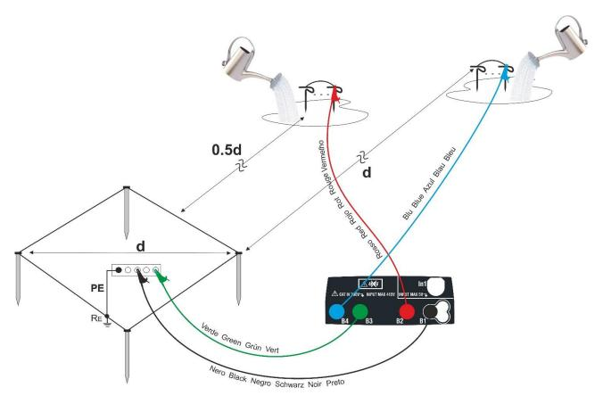
Fig. 48: Ground measurement for big-sized earth networks
