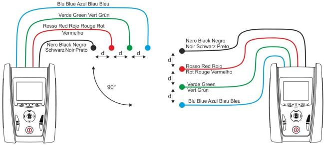
Fig. 49: Ground resistivity measurement
