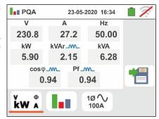
6. The screen to the side shows the real time values of electrical parameters in a Three phase balanced plant. For the meaning of the parameters refer to § 13.15. The symbols "\_\_\_\_\_" and "≠" show the type Inductive or Capacitive of the load respectively.
