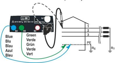
Fig. 22: P-PE/P-N measurement for 400V + PE (no N) systems by means of single cables
