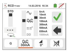
59 Ramp mode is fixed on the instrument. Move the reference of the lower sliding bar by selecting the type of display of the tripping current during the ramp test between the "NOM" or "REAL" options (see § 6.3)
