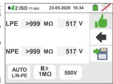
14 <u>For three-phase EVSE systems</u>, the measurement result of the <u>first L1PE test</u> is shown in the screen to the side. The values of the real test voltages are shown on the display
