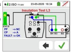
18 The measurement result of the **L3PE and NPE test** is shown in the screen to the side. The values of the real test voltages are shown on the display
