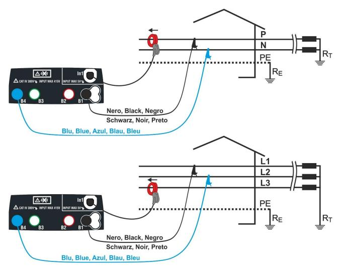
Fig. 37: Connection for measurement on Single phase installations
