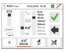
67 Ramp mode is fixed on the instrument. Move the reference of the lower sliding bar by selecting the type of display of the tripping current during the ramp test between the "NOM" or "REAL" options (see § 6.3).
