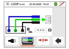
Insert the ZEROLOOP metallic accessory into the three banana connectors of the measurement cables (L-N-PE) or into the metal connectors of the Shuko plug (differently in the various types depending on the country of use) as shown in the following
