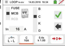
4. Touch the icon to zero the value in the In field and use the virtual keyboard to set the value of the RCD rated current within the values allowed by the instrument.
