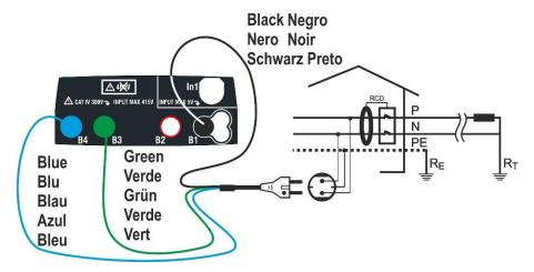
Fig. 12: Connection for single-phase 230V system by means of shuko plug
