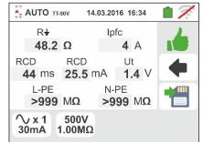
10 In case of **negative** result of the **NoTrip**; the auto test is automatically blocked, the symbol is shown and the screen to the side is displayed. Note red value of the contact voltage
