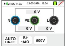
13 For single-phase EVSE systems, the measurement result is shown in the screen to the side. The values of the real test voltages are shown on the display. The symbol indicates the correct result of the measurement.
