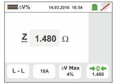
Connect the instrument to the final point of the main line being tested according to Fig. 34 or Fig. 35 in order to measure the **Z2** impedance at the end of line. The screen to the side is displayed. Note the previously measured Z1 (Offset) value displayed
