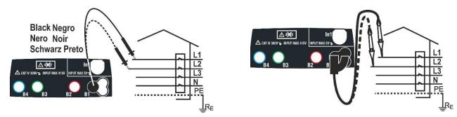
Fig. 24: Phase sequence check of 1T phases with terminal and remote lead
