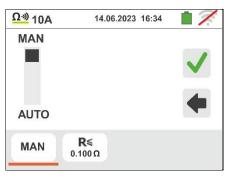
4. Touch the icon to reset the value in the "Ω" field and use the virtual keyboard to set the value of the maximum limit resistance used by the instrument for evaluating the continuity test in the field: 0.003Ω ÷ 0.500Ω in steps of 0.001Ω. Confirm your choice by returning to the previous screen
