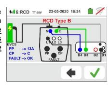
65 The test is performed by the instrument considering only General RCD of STD (G) type, type B/B+ or type DD and in Ramp mode ( ) 0°. Touch the second icon. The followed screen is shown on the display
