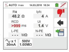
12 In case of **negative** result of the **RCD**, the auto test is automatically blocked, the symbol is shown and the screen to the side is displayed. Note red value of the tripping current
