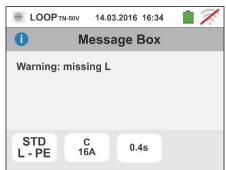
If the instrument detects the absence of the signal to terminal B4 (neutral conductor), it provides the warning screen shown to the side and blocks the execution of the tests.
