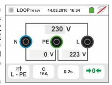
7. Press the **GO/STOP** key <u>for few seconds</u> or the **START** key on the remote lead. During this whole stage, do not disconnect the measuring leads of the instrument from the system under test.
