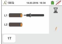
At the end of phase L1 acquisition, the instrument is in standby waiting for the signal on phase L2 and showing the symbol of "disconnected tip" as shown in the screen to the side.
