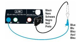
Fig. 7: Compensation of single cables and remote lead resistance
