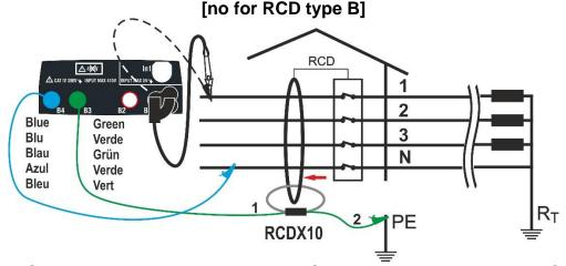
Fig. 17: Connection to earth leakage relay RCDs with optional accessory RCDX10
