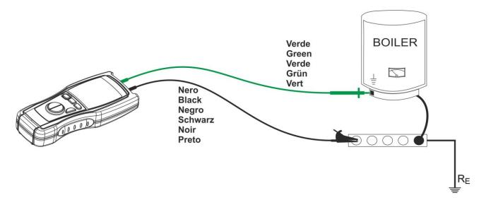
Fig. 9: Connection of the instrument's terminals during test
