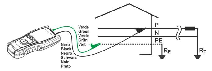
Fig. 3: Connection of the instrument's terminals
