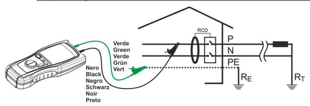
Fig. 11: Connection of the instrument's terminals during  $M\Omega$  test
