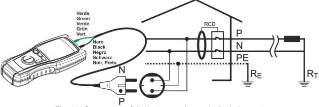
Fig. 13: Connection of the instrument's terminals during test
