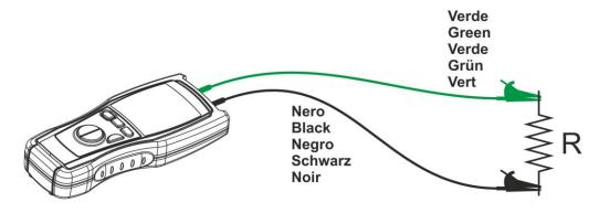
Fig. 5: Connection of the instrument's terminals
