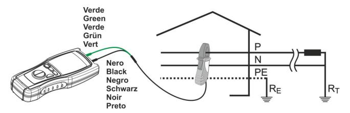
Fig. 4: Connection of the instrument's terminals
