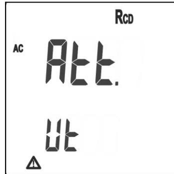
5. **With nominal current 30mA<sub>x5</sub>** if during measurement an excessive earth resistance is detected, such to prevent the instrument from generating the test current, the instrument does not perform the test and emits a prolonged sound to signal the anomalous situation. The screen beside is displayed for 5 seconds after which the instrument shows the default screen related to RCD test
