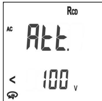
This can happen for example if the black cable is erroneously connected to the neutral conductor instead of the phase one. If a Shuko cable is used, rotate the plug and repeat the test
