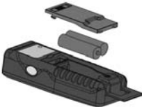
Fig. 14: Replacement of the internal battery
