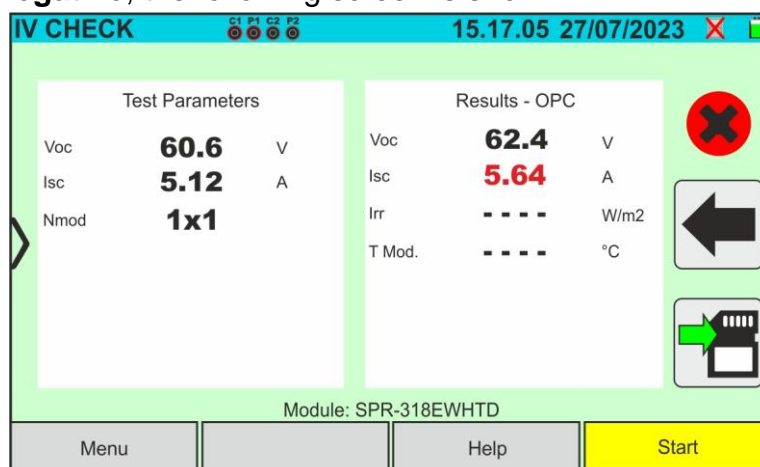
Fig. 52: Example of a negative IVCK test result - OPC values
