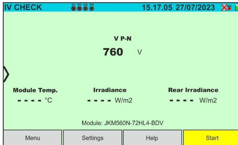
Fig. 74: IVCK test screen with SOLAR03 in synchronous recording on Bifacial modules
