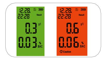
5. If the result is ≥0.8g/L, the message "Danger" is shown on the display, the background turns "red" and the buzzer emits a warning sound
