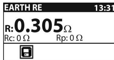
Fig. 26: Result screen of earth resistance measurement
