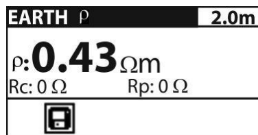
Fig. 29: Result screen of ground resistance measurement
