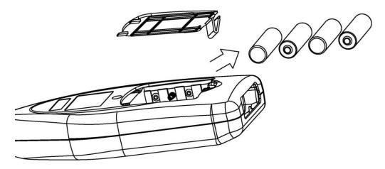
Fig. 55: Replacement of internal batteries
