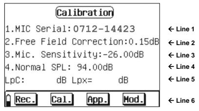
Fig. 35: Initial screen of calibration section
