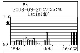
Fig. 52: Graphic display of 1/3 spectrum analysis
