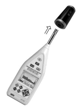
Fig. 36: Insertion of the calibrator HT151 into the instrument
