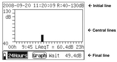
Fig. 17: Screen of graphic display in 24Hours mode
