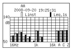
Fig. 49: Graphic display of 1/1 spectrum analysis
