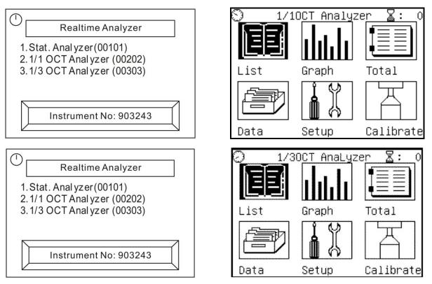
Fig. 22: Initial screens for analysis in 1/1 and 1/3 octave band
