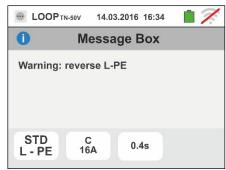
8. If the instrument detects a danger voltage on PE conductor, it does not carry out the test and displays a screen like the one to the side. This message can also appair in case of an insufficient pressure of the **GO/STOP** key
