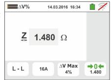
13 Connect the instrument to the final point of the main line being tested according to Fig. 34 or Fig. 35 in order to measure the **Z2** impedance at the end of line. The screen to the side is displayed. Note the previously measured Z1 (Offset) value displayed
