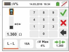
8. Touch the icon to zero the value in "A" field and use the virtual keyboard to set the value of rated current of protection device in the range **1A** to **9999A**. Confirm selection and go back to the previous screen.
