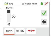
3. Touch the icon to zero the value in the Timer field and use the virtual keyboard to set the value in seconds between 1s and 99s. Confirm the choice by going back to the initial measurement screen.
