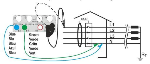
Fig. 14: Connection three phase 4-wire (no PE), single cables, remote lead (**no RCD B/B+ type**)
