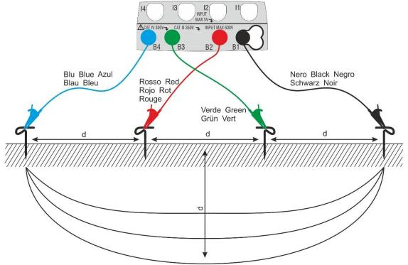
Fig. 30: Ground resistivity measurement
