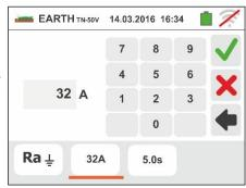
Touch the icon to zero the value in the "s" field and use the virtual keyboard to set the value of the time for fault elimination t (declared by the Energy distribution board) between **0.04s** and **10s**.
