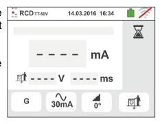
10 At the end of the test, if the tripping current is within the values of the table in the relevant §, the instrument displays the symbol to indicate the positive outcome of the test and displays a screen like the one to the side.
