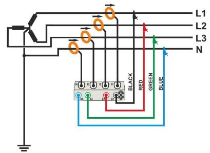
Fig. 37: Connection for measurement on Three-phase system 3φ-4WIRES
