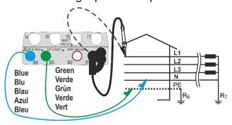
Fig. 19: L-N/L-PE test for three-phase systems by means of single cables and remote lead
