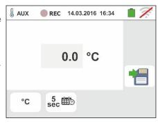
2 Move the slide bar reference to select the type of measurement among the options: °C (temperature in Celsius degrees), °F (temperature in Fahrenheit degrees), Lux(20) (illuminance with 20Lux capacity), Lux(2k) (illuminance with 2kLux capacity), Lux(20k) (illuminance with 20kLux capacity) ,%RH (relative humidity), mV (measurement of DC voltage up to 1V)
