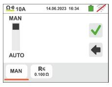
Touch the icon to reset the value in the " $\Omega$ " field and use the virtual keyboard to set the value of the maximum limit resistance used by the instrument for evaluating the continuity test in the field:  $0.003\Omega \div 0.500\Omega$  in steps of  $0.001\Omega$ . Confirm your choice by returning to the previous screen
