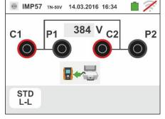
5. The standard (STD) short-circuit current is shown in the upper part of the display.
