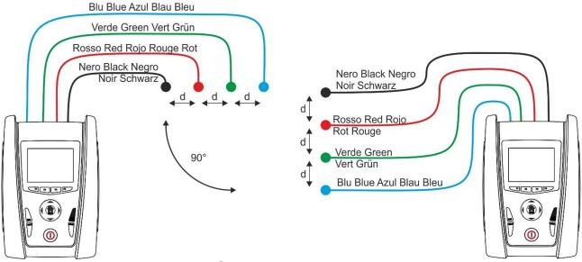
Fig. 55: Ground resistivity measurement
