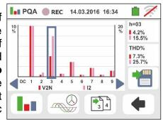
harmonic order. Press the **SAVE** button or touch the icon to save the measurement on the display as instantaneous snapshot (see § 7.1). Touch the op icon to go back to the main screen of RMS values
