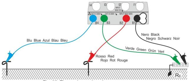
Fig. 27: Three-wire earth resistance measurement
