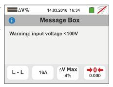
If the instrument detects the absence of the signal to terminal B1 (phase conductor), it provides the warning screen shown to the side and blocks the execution of the tests
