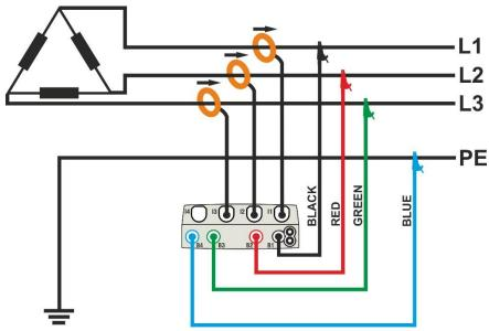
Fig. 39: Connection for measurement on Three-phase system 3φ-ARON
