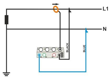
Fig. 36: Connection for measurement on single-phase 1φ-2WIRES
