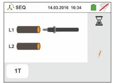
At the end of phase L1 acquisition, the instrument is in standby waiting for the signal on phase L2 and showing the symbol of "disconnected tip" as shown in the screen to the side.
