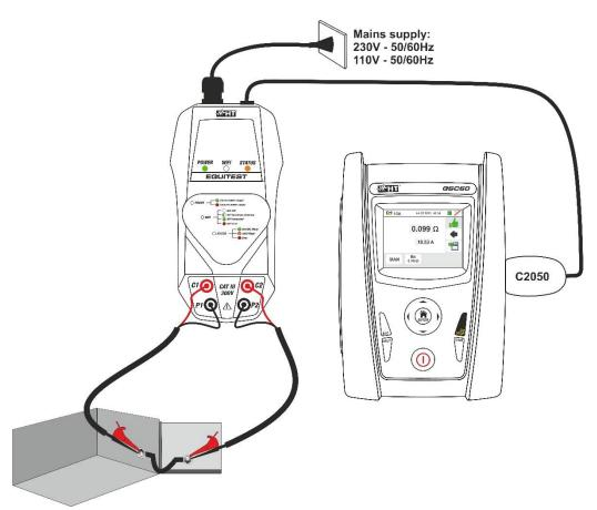
Fig. 33: Continuity test by means of EQUITEST accessory
