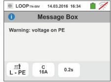
If the instrument detects a voltage VN-PE>50V (or >25V depending on the selection), it does not carry out the test and displays a screen like the one to the side
