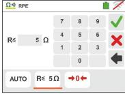
Confirm the choice by going back to the initial measurement screen. Note the presence of the set limit value.
