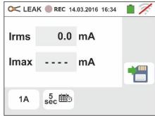
2. Touch the arrow keys or to set the full scale value of the selected HT96U clamp in the 1A ÷ 3000A range. Press and hold the keys for a quick selection of values
