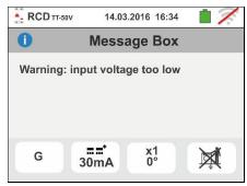
15 For test on earth leakage relay RCD if the value set for the rated current of the protection device is out of the allowed range, the instrument provides the warning screen shown to the side and stops the tests. Change the value of the rated current of the protection device
