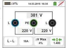
14 Press the **GO/STOP** key on the instrument to measure the Z2 impedance and complete the ΔV% voltage drop measurement. During this whole stage, do not disconnect the measuring leads of the instrument from the system being tested
