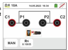
Connect the EQUITEST to the main supply supply and note the switch on of LED greenPOWER. Connect the accessory to the instrument through the C2050 cable. The screen alongside is shown on the display with the accessory connected regularly
