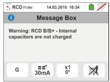
14 For only RCD type B/B+ if the instrument detects a input voltage VL-N <190V, it provides the warning screen shown to the side and blocks the test. Chech the values of the voltages on the installation
