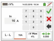
9. Touch the icon to zero the value in the "%" field and use the virtual keyboard to set the value of  $\Delta V\%$  in the range **1%** to **99%**.
