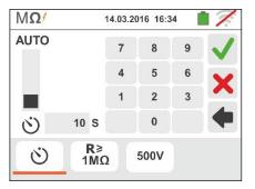
Touch the icon "R≥xxΩ" to set the minimum limit value of the insulation resistance on which the instrument makes the comparison with the measured value. The screen to the side appears on the display.
