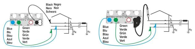
Fig. 18: L-N/L-PE measure for single-phase/two-phase with cables and remote lead
