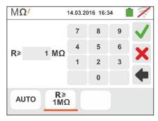
5. Touch the "xxxxV" icon to set the test DC voltage in the insulation measurement. The screen to the side appears on the display.
