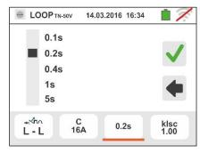
Touch the icon to zero the value in the field and use the virtual keyboard to set the calculation coefficient of the short circuit current **Isc** within the values allowed by the instrument
