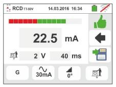
11 At the end of the test, if the tripping current is not within the values of the table in the relevant §, the instrument displays the symbol to indicate the negative outcome of the test and displays a screen like the one to the side.
