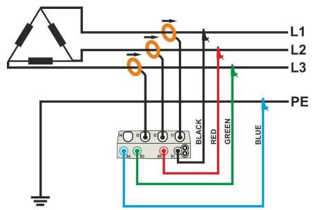
Fig. 38: Connection for measurement on Three-phase system 3φ-3WIRES
