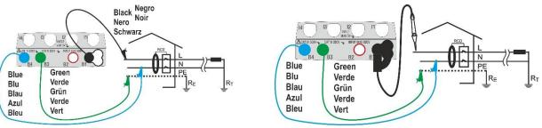
Fig. 12: Connection for single-phase system with single cables and remote lead
