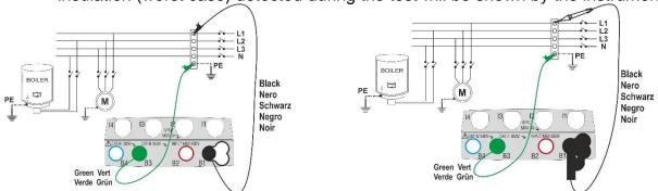
Fig. 8: Insulation test by means of single cables and remote lead
