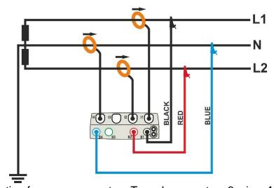
Fig. 44: Connection for measurement on Two-phase system 3-wires 1φ- CentrePoint
