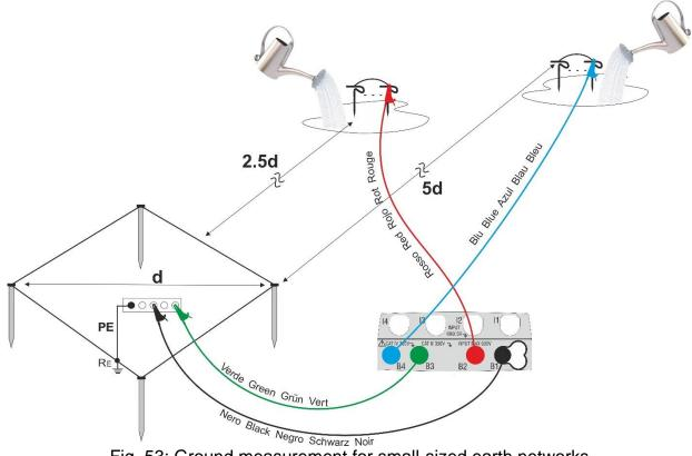
Fig. 53: Ground measurement for small-sized earth networks
