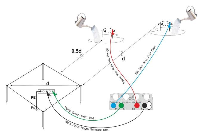
Fig. 54: Ground measurement for big-sized earth networks
