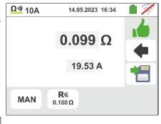
7. At the end of the test, if the measured resistance value is higher than the set limit, the screen to the side is shown on the display. The value is shown in red and the symbol indicates the non-ok result of the measurement. The indication ">1.999Ω" indicates the out of range of the EQUITEST accessory
