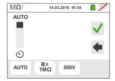
Touch the icon to zero the value in the Timer field and use the virtual keyboard to set the value in seconds between 1s and 999s. Confirm the choice by going back to the initial measurement screen.
