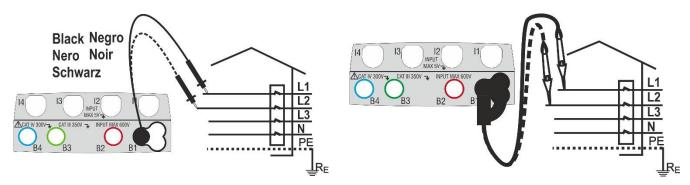
Fig. 23: Phase sequence check of 1T phases with terminal and remote lead
