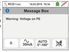
10 If the instrument detects a dangerious contact voltage Ut (over the set limit 25V or 50V) in the starting pre-test, it provides the warning screen shown to the side and blocks the execution of the tests. Check the PE conductor and earth plant efficiency
