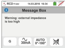
13 For only RCD type B/B+ if the instrument is not able to provide for the charging of the internal capacitors of the RCD, it provides the warning screen shown to the side and blocks the test. Check that the VL-N voltage should be more than 190V
