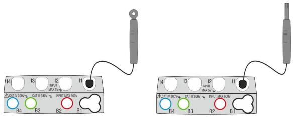
Fig. 32: Measurement of environmental parameters through external probes
