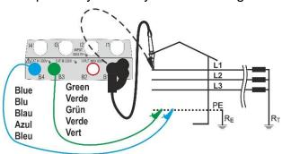
Fig. 21: L-PE/L-N test for three-phase systems (no N) by means of single cables and remote lead
