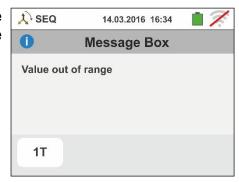
3. If the instrument detects an input voltage frequency exceeding the allowed full scale, it will display a screen like the one to the side.
