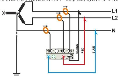
Fig. 43: Connection for measurement on Two-phase system 3-wires **3**φ**-2EI.** ½
