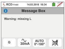
4. If the instrument detects the absence of the signal to terminal B4 (neutral conductor), it provides the warning screen shown to the side and blocks the execution of the tests.
