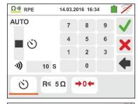
4. Touch the icon "R≤xxΩ" to set the maximum limit value of the resistance on which the instrument makes the comparison with the measured value. The screen to the side appears on the display. Touch the value in the "R≤" field. Use the virtual keyboard to set the value between  $1\Omega$  and  $99\Omega$ .
