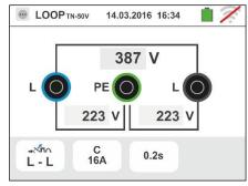
7. Press the **GO/STOP** key for 2s or the **START** key on the remote lead. During this whole stage, do not disconnect the measuring leads of the instrument from the system under test.
