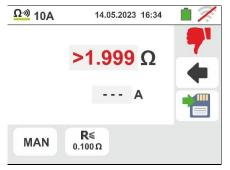
8. <u>In the AUTO measurement</u>, the instrument goes into standby and displays the screen to the side after performed a test.
