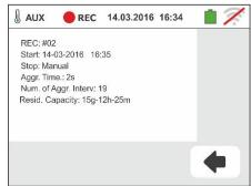
9. Press **GO/STOP** key to stop recording; the instrument automatically saves the result in its memory (see § 7.1.3). The message to the side is shown.
