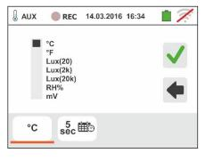
Touch the sec icon to set the parameters of recording. The followed screen is shown
