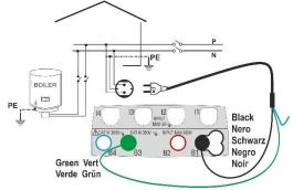
Fig. 9: Insulation test by means of shuko plug
