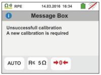
3. In case the instrument detects that the calibrated resistance is higher that the measured resistance, the instrument gives out a long sound and displays a screen like the one to the side. The ticon is shown on the display to indicate the calibration reset value.
