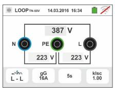
8. Press the **GO/STOP** key for 2s or the **START** key on the remote lead. During this whole stage, do not disconnect the measuring leads of the instrument from the system under test.
