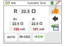
2. If in  $\longrightarrow 0 \longleftarrow$  mode the instrument detects a resistance higher than  $2\Omega$  at its terminals, it resets the offset value and displays a screen like the one to the side. The  $\longrightarrow 0 \longleftarrow$  icon is shown on the display to indicate the calibration reset value (i.e. performing the operation with open terminals).
