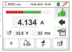
11 At the end of the test, if the tripping current is higher to the set value, the instrument displays the symbol to indicate the negative outcome of the test and displays a screen like the one to the side.
