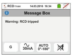
9. If the instrument detects a dangerious voltage on PE conductor it provides the warning screen shown to the side and blocks the execution of the tests. Check the PE conductor and earth plant efficiency. This message can also appair in case of an insufficient pressure of the GO/STOP key
