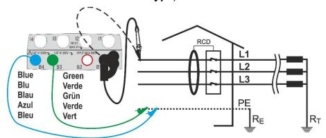
Fig. 15: Connection for a three phase 3-wire (no N) single cables, remote lead (no RCD B
