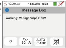
12 If the instrument detects in the input terminals a too high external impedance such that it can not provides the nominal current, it provides the warning screen shown to the side and blocks the test. Disconnect the possible loads downstream the LCD before perform the test
