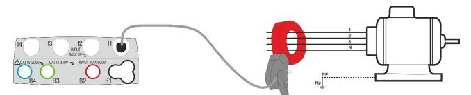
Fig. 25: Indirect measurement of leakage current in three-phase systems
