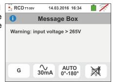
If the voltage between inputs B1 and B4 and inputs B1 and B3 is lower than 100V, the instrument provides the warning screen shown to the side and blocks the execution of the tests.
