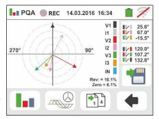
In the bottom part of the display there are the "Rev" and "Zero" indications associated with the unbalance of input voltages (see § )
