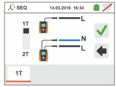
3. Insert the blue and black connectors of the single cables in the corresponding input terminals of the instrument B4, B1 (2T measurement). Insert in the free end of the cables the corresponding alligator clips or tips. It is also possible to use the remote lead by inserting its multipolar connector into the input lead B1. Connect the alligator clips, the tips or the remote lead to phase L1 and N according to Fig. 23 and Fig. 24.
