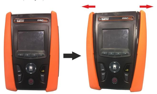
Fig. 46: Remove lateral half-shells
