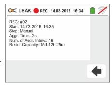
10 Press **GO/STOP** key to stop recording; the instrument automatically saves the result in its memory (see § 7.1.3). The message to the side is shown. ✓ LEAK ● REC 14.03.2016 16:34
