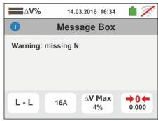
If the instrument detects the absence of the signal to terminal B3 (PE conductor), it provides the warning screen shown to the side and blocks the execution of the tests.
