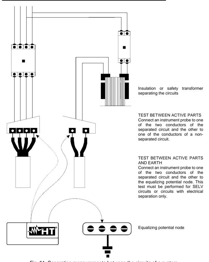
Fig. 51: Separation measurements between the circuits of a system
