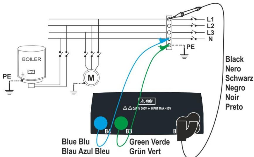
Fig. 14: Insulation between L-N-PE with single cables and remote switch probe (MAN and AUTO)
