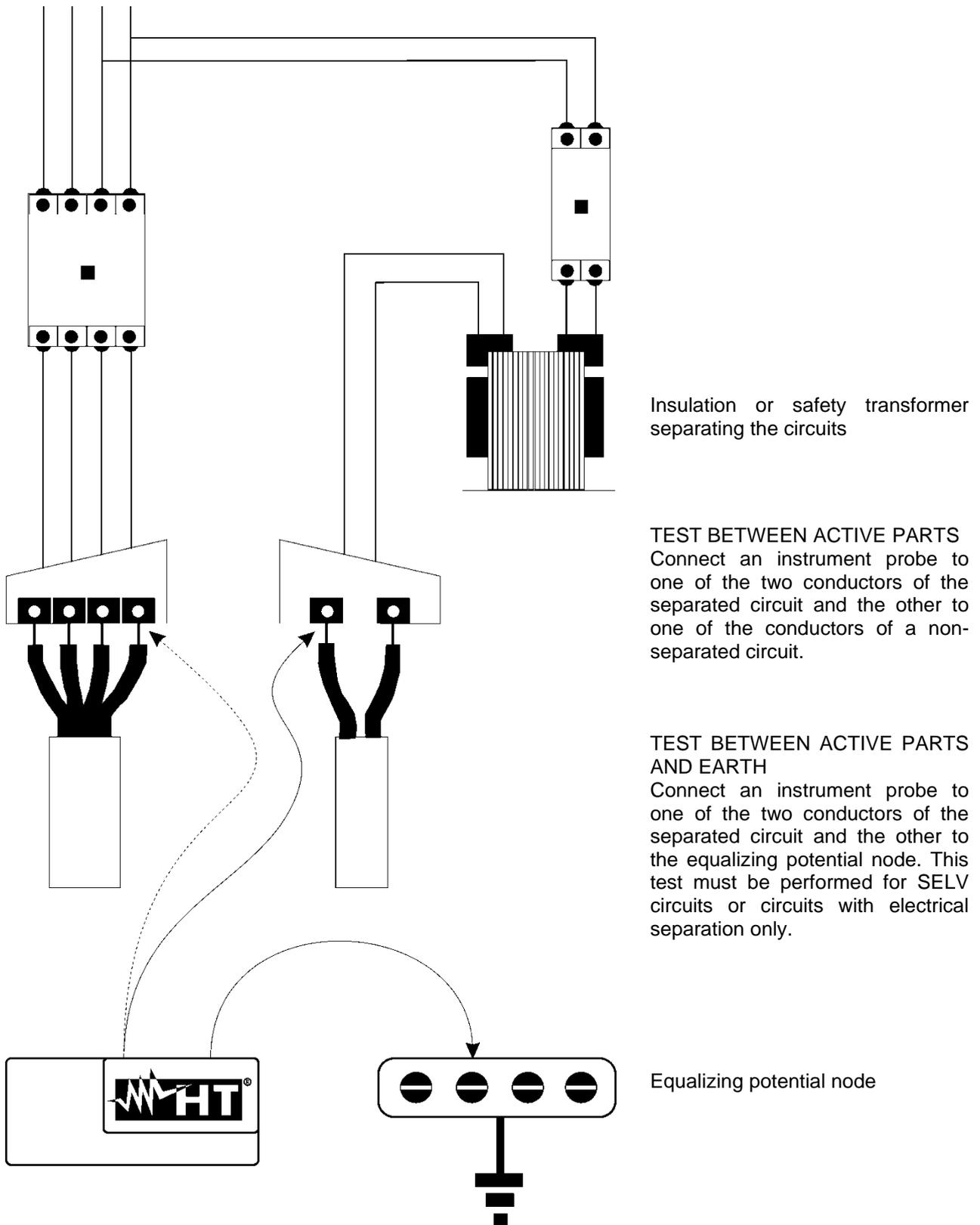
Fig. 40: Separation measurements between the circuits of a system
