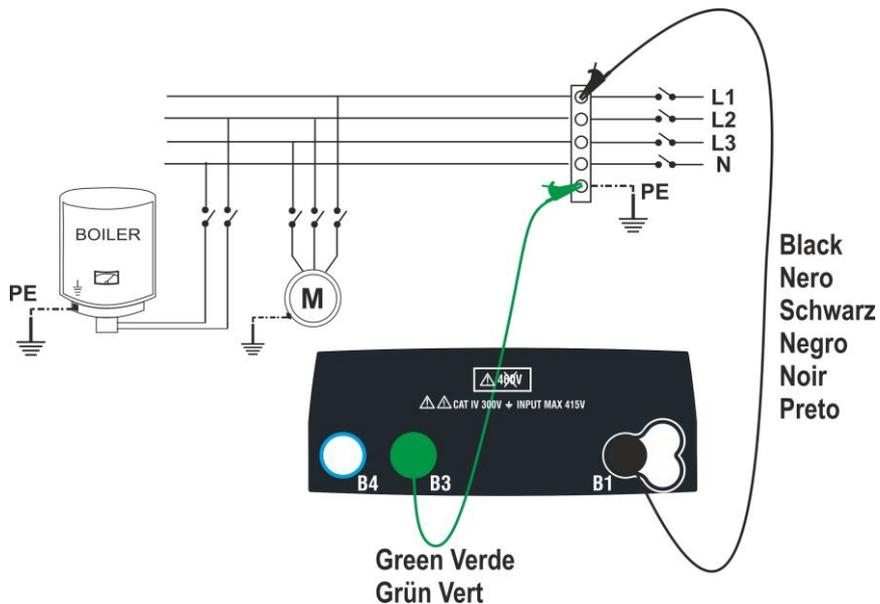
Fig. 17: Insulation between L-PE by means of single cables (TMR mode)
