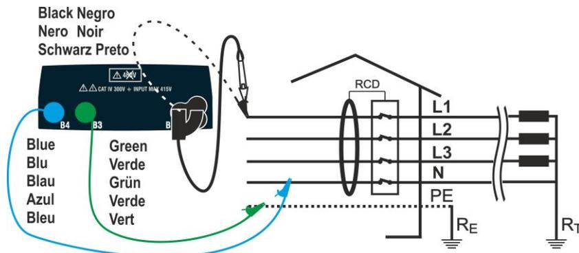
Fig. 21: Connection for three-phase L1-L2-L3-N system by means of single cables and remote switch probe
