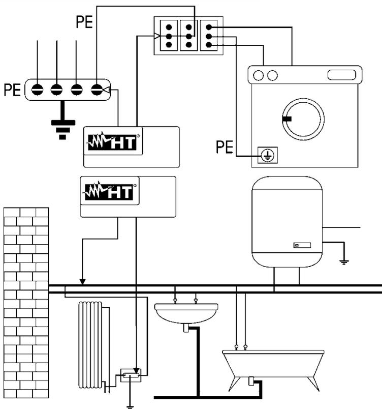
Connect one of the test leads to the protective conductor of the socket and the other to the equalizing potential node of the earth installation.
