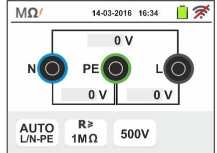
2. Move the slide bar reference in the positions "AUTO" (Automatic mode) or "⌚" (Timer mode). Move the right slide bar reference in the "L/N-PE" position. Confirm the choice by going back to the previous screen.
