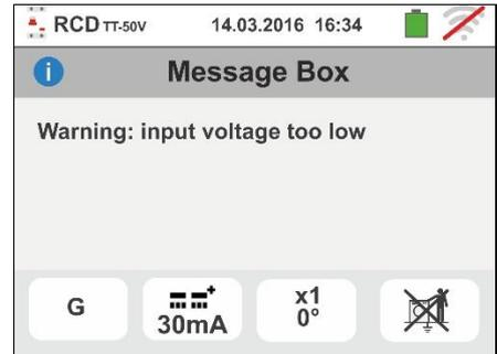
15 **For test on earth leakage relay RCD** if the value set for the rated current of the protection device is out of the allowed range, the instrument provides the warning screen shown to the side and stops the tests. Change the value of the rated current of the protection device
