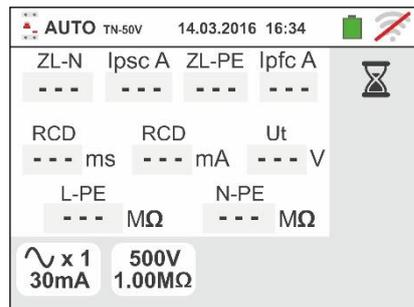
8. In case of **positive** result of the three test sequentially performed as **NoTrip<sup>+</sup>** (**ZL-N** and **ZL-PE<199Ω**), **RCDX1** (see § 13.4) and **MΩ L/N-PE** the symbol is shown and the screen to the side is displayed by the instrument
