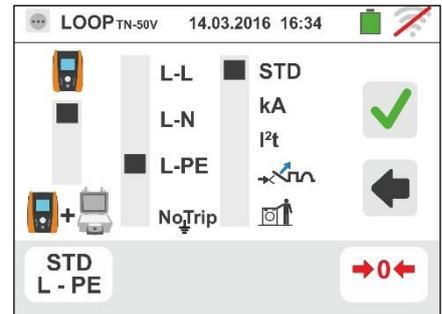
Touch the icon in the lower right corner to set the maximum tripping current expressed in "kA" that the protection must interrupt. The following screen appears on the display:
