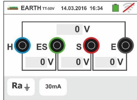
Touch the first icon in the lower left corner to set the measuring mode. The following screen appears on the display:
