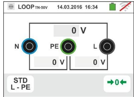
6. The value of the test leads/Shuko plug resistance various plugs is maintained by the instrument up to the reset operation performed by the user (for example for the insertion of cables with different lengths). To perform the reset of saved calibration value, touch the
