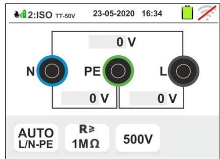
13 For single-phase EVSE systems, the measurement result is shown in the screen to the side. The values of the real test voltages are shown on the display. The
