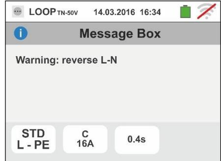
7. If the instrument detects that the phase and PE leads are inverted, it does not carry out the test and a screen similar to the one reported to the side is displayed. Check the connection of measuring cables.
