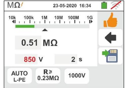
7. **In the L/N-PE test** if in one of both test the instrument measures a resistance higher than the set limit value but for which it is not able to generate the rated voltage, the screen to the side is displayed.
