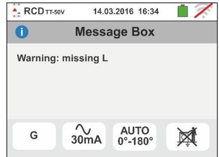
4. If the instrument detects the absence of the signal to terminal B4 (neutral conductor), it provides the warning screen shown to the side and blocks the execution of the tests.
