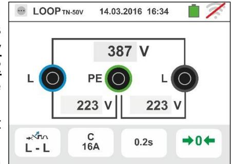
7. Press the **GO/STOP** key for few seconds or the **START** key on the remote lead. During this whole stage, do not disconnect the measuring leads of the instrument from the system under test.
