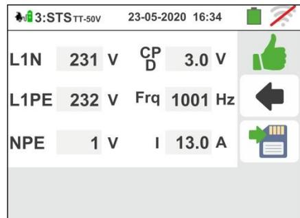
37 If the test fails, the screen like the one on the side is shown on the display. The incorrect value of the parameter is shown in red and the symbol
