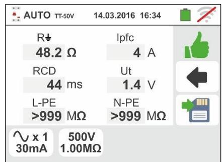
9. In case of **positive** result of the three test sequentially performed as **NoTrip** (see § 13.8), **RCD** (see § 13.4) and **MΩ L/N-PE** the symbol is shown and the screen to the side is displayed by the instrument.
