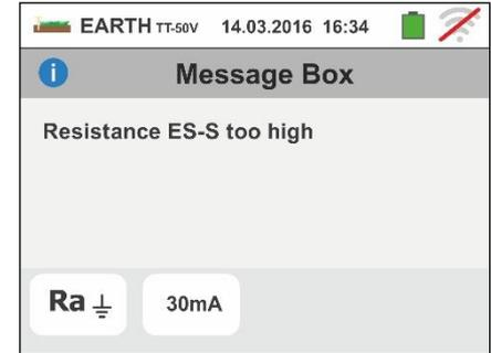
3. When starting a measurement, the instrument checks the continuity of measuring cables. **If the ampermetric circuit (blue cable H and black cable E) is interrupted or its resistance value is too high**, the instrument displays a screen similar to the one on the side.
