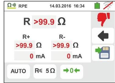
12. At the end of the test in the “
