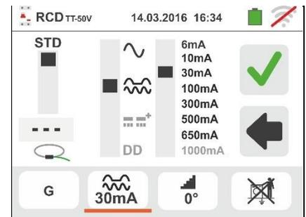
59 **Ramp mode
