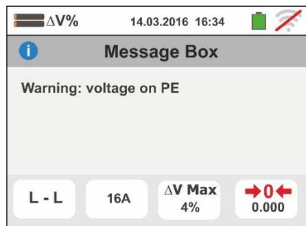
9. If the instrument detects a voltage  $V_N-PE > 50V$  (or  $> 25V$  depending on the selection), it does not carry out the test and displays a screen like the one to the side
