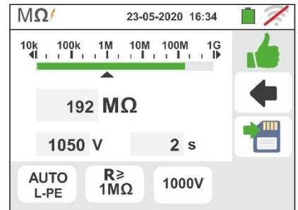
11. At the end of the test, if the value of the measured resistance is lower than the set limit, the screen to the side is shown on the display.
