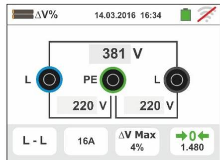
10 Press the **GO/STOP** key on the instrument to measure the Z2 impedance and complete the  $\Delta V\%$  voltage drop measurement. During this whole stage, do not disconnect the measuring leads of the instrument from the system being tested
