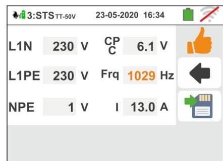
33 If the test fails, the screen like the one on the side is shown on the display. The incorrect value of the parameter is shown in red and the symbol
