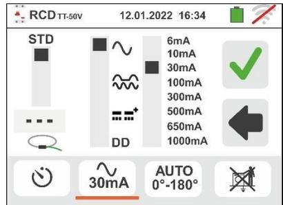
5. Touch the icon
