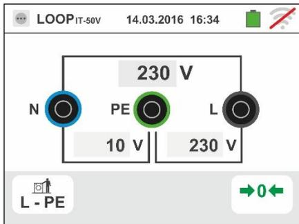
4. Press the **GO/STOP** key for few seconds or the **START** key on the remote lead. During this whole stage, do not disconnect the measuring leads of the instrument from the system under test.
