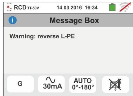
8. If the differential switch being tested trips during the preliminary checks (performed automatically by the instrument before executing the selected test), the instrument does not carry out the test and displays a screen like the one to the side. Check that the IdN set value is consistent with the differential switch in question and that all loads connected downstream of it are disconnected.
