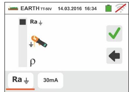
Touch the second icon in the lower left corner to set the tripping current of the differential switch (**TT and IT systems**). The following screen appears on the display:
