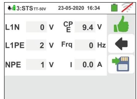
45 If the test fails, the screen like the one on the side is shown on the display. The incorrect value of the parameter is shown in red and the symbol indicates the non-ok result of the measurement. Press again the **GO/STOP** key to repeat the test
