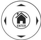
◀ ▶ ▲ ▼ keys to move the cursor through the different screens in order to select the desired programming parameters
