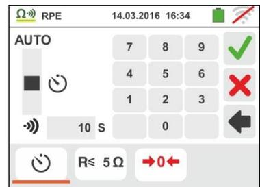
4. Touch the icon "R≤xxΩ" to set the maximum limit value of the resistance on which the instrument makes the comparison with the measured value. The screen to the side appears on the display.
