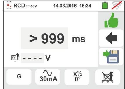
Press the **SAVE** button or touch the
