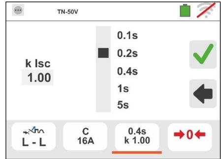
6. Touch the icon to zero the value in the field and use the virtual keyboard to set the calculation coefficient of the short circuit current **Isc** within the values allowed by the instrument
