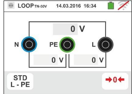
2. Move the left slide bar reference by selecting the icon to execute the measurement only with the instrument or the icon to execute the measurement with the instrument + optional accessory IMP57 (see § 6.4.13). Move the central slide bar reference by selecting the "L-L, L-N or L-PE" options. Move the right slide bar reference by selecting the "STD" option. Confirm the choice by going back to the previous screen.
