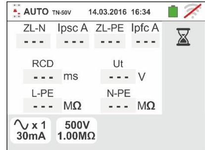
7. Press the **GO/STOP** key for few seconds or the **START** key on the remote lead. During this whole stage, do not disconnect the measuring leads of the instrument from the system under test. In case of **RCD tripping current measurement** selection the screen to the side appears on the display when the hourglass icon indicates the performance of the test
