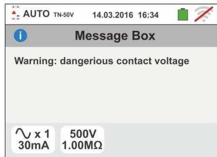
11 If the instrument detects a voltage value higher than 10V at its terminals, it does not carry out the L/N-PE insulation test, gives out a long sound and the screen reported here to the side is displayed
