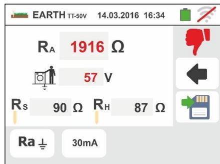
Note the presence of the measurement result highlighted in red.
