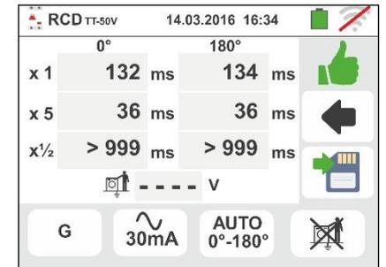
13 At the end of the test, if the tripping time of a test does not comply with what is indicated in Table 6 (see § 13.4).
