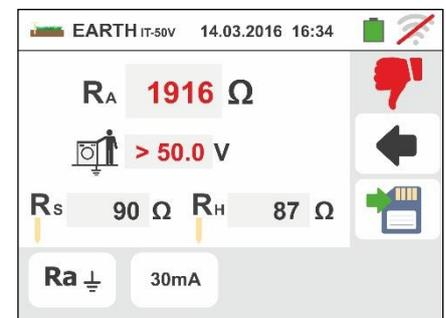
9. For **earth resistance measurement in TN systems**, in case of **positive** result (measured value LOWER than set limit value), the screen to the side is displayed by the instrument. It contains also the value of contact resistance of the voltage probe ( $R_s$ ) and the value of contact resistance of the current probe ( $R_h$ ).
