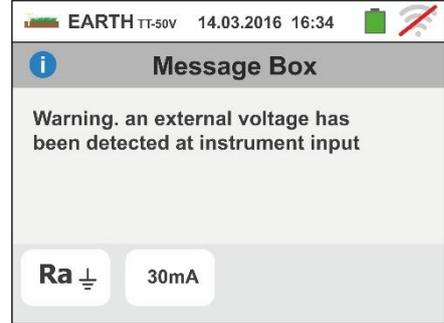
2. When starting a measurement, the instrument checks the continuity of measuring cables. **If the voltmetric circuit (red cable S and green cable ES) is interrupted or its resistance value is too high**, the instrument displays a screen similar to the one on the side.
