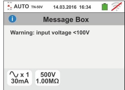
3. If the instrument detects the absence of the signal to terminal B1 (phase conductor), it provides the warning screen shown to the side and blocks the execution of the tests
