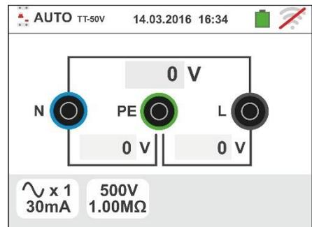
2. Move the left slide bar reference by selecting the waveform of the differential switch between the options: (type AC),  (type A/F),  (type B/B+). Move the second slide bar reference by selecting the desired rated current of the differential switch between the options: **6mA, 10mA, 30mA, 100mA, 300mA** Move the third slide bar reference by selecting the type of the test between the following options:
