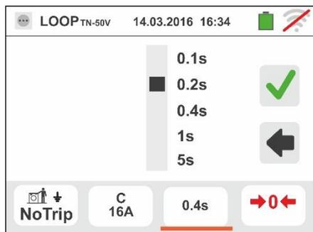
6. If possible, disconnect all loads connected downstream of the measured point, as the impedance of these users could distort the test results. Perform the preliminary calibration of the test leads as described in § 6.4.2 Connect the alligator clips or the remote lead to the electrical mains according to Fig. 18, Fig. 19, Fig. 20 and Fig. 22 in the farthest possible point respect the protection on test.
