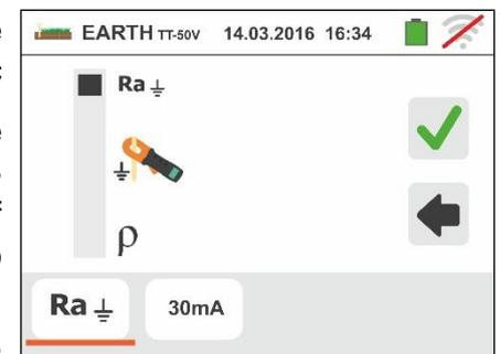
3. Move the slide bar reference in the position corresponding to the value of the tripping current of the RCD differential switch as shown in the screen to the side. On the basis of this selection and the value of contact voltage (25V or 50V), the instrument performs the calculation of the limit value of earth resistance (see § 13.12) that will compare with the measured value in order to provide the final positive or negative result of the measurement.
