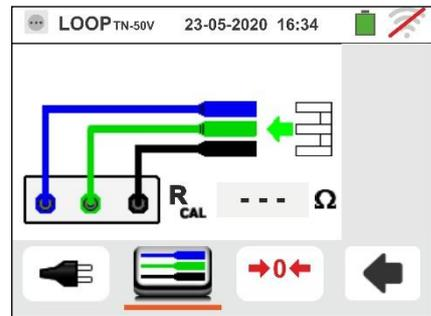
3. Insert the **ZEROLOOP** metallic accessory into the three banana connectors of the measurement cables (L-N-PE) or into the metal connectors of the Shuko plug (differently in the various types depending on the country of use) as shown in the following
