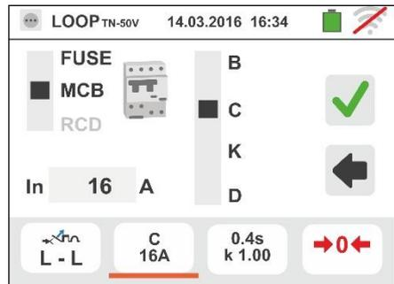
4. Touch the
