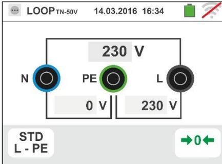
6. The value of the assumed short-circuit current (I<sub>sc</sub>) is shown in the upper part of the display, while the Line/Loop Z<sub>PE</sub> impedance is shown at the bottom of the display. Press the **SAVE** button or touch the icon to save the measurement (see § 7.1).
