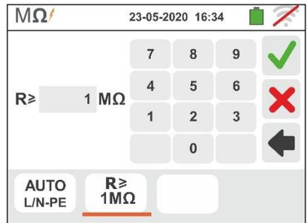
4. Touch the "xxxxV" icon to set the test DC voltage in the insulation measurement. The screen to the side appears on the display.
