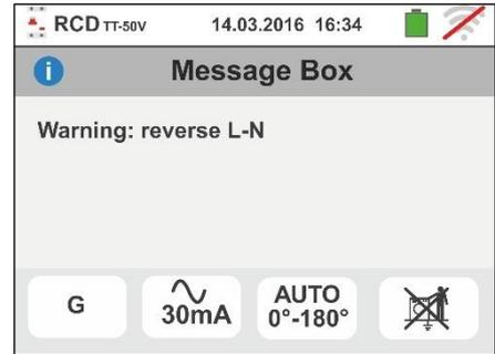
7. If the instrument detects that the phase and PE leads are inverted, it does not carry out the test and a screen similar to the one reported to the side is displayed. Check the connection of measuring cables.
