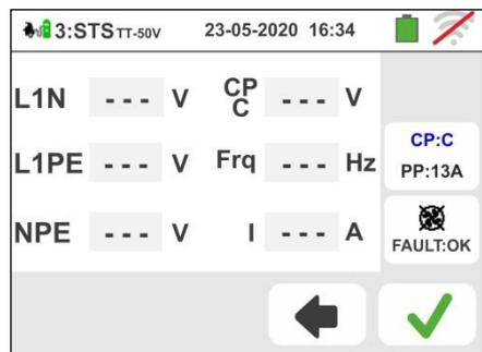
32 The result of the measurement is shown in the screen to the side. The symbol indicates the correct result of the measurement. The symbol also indicates a positive result of the measurement but with values outside the limits present in the Table 4.
