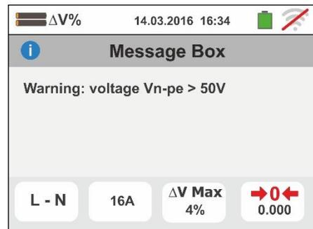
10. If during the measurement the instrument detects an end of line impedance value lower than the initial line impedance value it does not carry out the test and a screen similar to the one reported to the side is displayed. Check the status of the main line being tested
