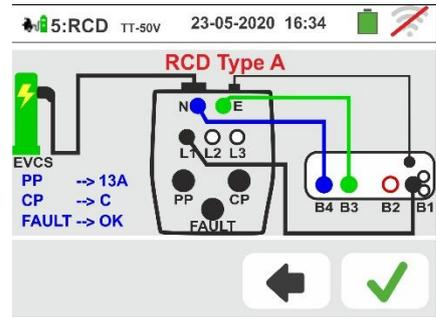
57 The test is performed by the instrument considering **only General RCD of STD (G) type, type A/F and in Ramp mode (
