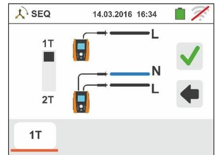
3. Insert the blue and black connectors of the single cables in the corresponding input terminals of the instrument B4, B1 (2T measurement). Insert in the free end of the cables the corresponding alligator clips or tips. It is also possible to use the remote lead by inserting its multipolar connector into the input lead B1. Connect the alligator clips, the tips or the remote lead to phase L1 and N according to Fig. 24 and Fig. 25.
