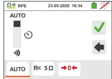
3. Touch the
