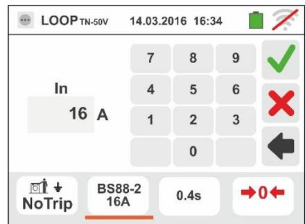
5. Move the slide bar reference by selecting the protection tripping time between the options: **0.4s**, **5s**
