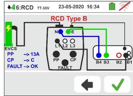
65 The test is performed by the instrument considering **only General RCD of STD (G) type, type B/B+ or type DD and in Ramp mode (📈) 0°**. Touch the second icon. The followed screen is shown on the display
