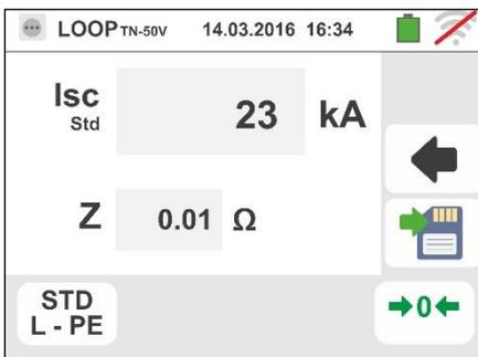
The Standard (Std) assumed short-circuit current (I<sub>sc</sub>) is calculated using the following formula:
