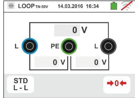
2. Move the left slide bar reference by selecting the icon to execute the measurement only with the instrument or the icon to execute the measurement with the instrument + optional accessory IMP57 (see § 6.4.13). Move the central slide bar reference by selecting the “L-L”, “L-N” or “L-PE” options (for TN systems only). Move the right slide bar reference by selecting the “kA” option.
