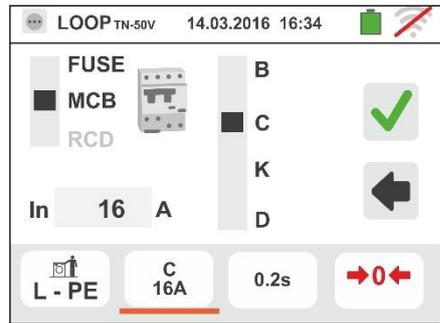
4. Touch the
