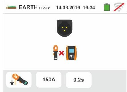
2. Connect the clamp T2100 by inserting the connector into input **In1** of the instrument. Turn the clamp on and put it in "RS232" mode (see the user manual of the clamp). The symbol appears on the display of the clamp. **In these conditions, the instrument-clamp group is ready to perform the measurements.** The following screen is shown on the display by the instrument.
