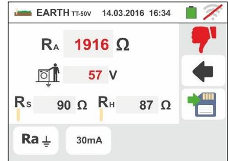
8. For **earth resistance measurement in IT systems**, in case of **negative** result (see § 13.9), the screen to the side is displayed by the instrument. It contains the value of contact voltage in the secondary display, the value of contact resistance of the voltage probe ( $R_s$ ) and the value of contact resistance of the current probe ( $R_h$ ).
