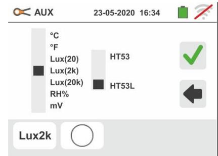
3. **If the HT53L probe is used**, select the color of the LED source under test from the options: (standard white light source) or (LED/colored source) as shown in the screen to the side
