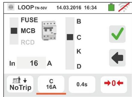
4. Touch the icon to zero the value in the In field and use the virtual keyboard to set the value of the nominal current of the protection within the values allowed by the instrument (see § 6.4.5)
