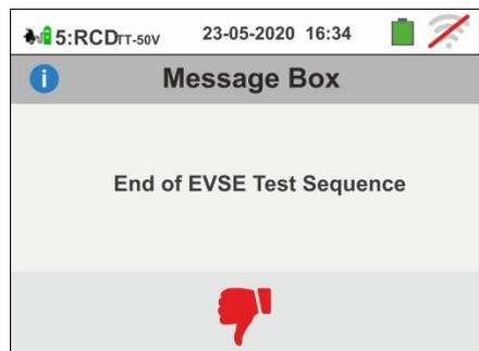
Test 6 → Test of RCD type B/B+ or DD of EVSE system
