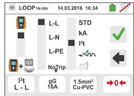
3. Move the slide bar reference by selecting the type of protection (Fuse of type **gG** or **aM** or magnetothermal MCB in curve **B**, **C**, **K**, **D**).
