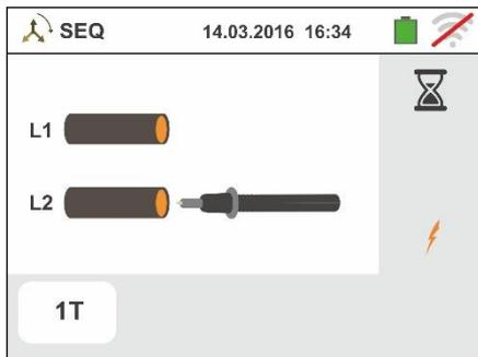
8. At the end of the test, if the detected phase sequence is correct, the instrument displays a screen like the one shown to the side (result "1-2-3").
