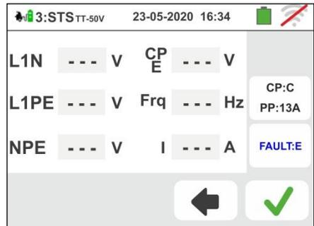
44 The result of the measurement is shown in the screen to the side. The symbol indicates the correct result of the measurement. The symbol also indicates a positive result of the measurement but with values outside the limits present in the Table 4
