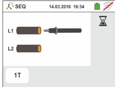
5. Once the correct voltage recognized, the ⚡ symbol is shown on the display. The instrument gives out a long sound until input voltage is present.
