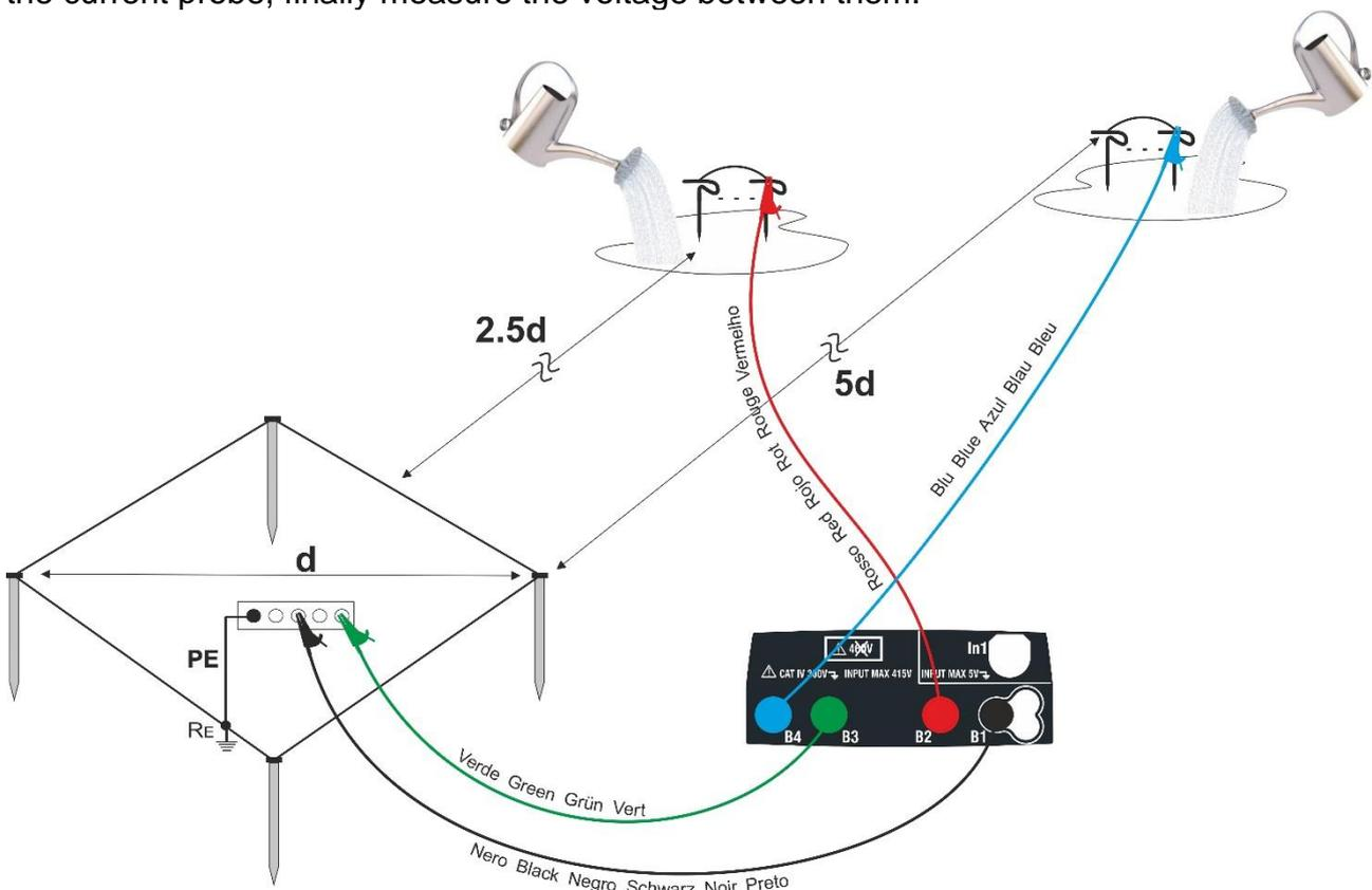
Fig. 47: Ground measurement for small-sized earth networks
