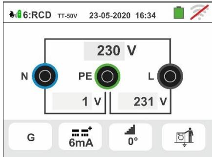
66 Move the third slide bar reference by selecting the desired rated current of the differential switch between the options: **6,10, 30, 100, 300mA (type B/B+) or 6mA (type DD)**
