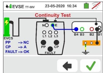
7. The RPE test is performed by the instrument **only in AUTO mode**. Set the limit threshold value and calibrate the measurement cables as shown in § 6.1
