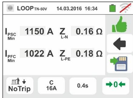
8. (**Z<sub>L-PE</sub> HIGHER to limit impedance relative to protection device within the specified time** – see § 13.7), the screen to the side is displayed by the instrument. Press the **SAVE** button or touch the
