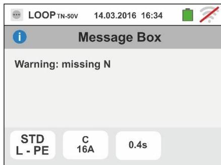
5. If the instrument detects the absence of the signal to terminal B3 (PE conductor), it provides the warning screen shown to the side and blocks the execution of the tests.
