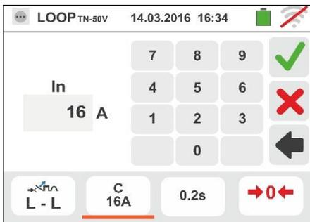
5. Move the slide bar reference by selecting the protection tripping time between the options: **0.1s**, **0.2s**, **0.4s**, **1s**, **5s** (all countries except AUS/NZ and UK), **0.4s**, **5s** (option L-PE, Fuse protection for AUS/NZ and UK) and **0.4s** (option L-PE, MCB protection for AUS/NZ).
