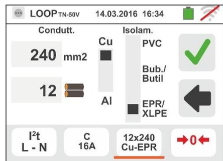
Move the central slide bar reference by selecting the type of conductor. The available options are **Cu** (Copper) and **Al** (Aluminum).
