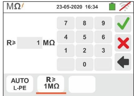
5. Touch the "xxxxV" icon to set the test DC voltage in the insulation measurement. The screen to the side appears on the display.
