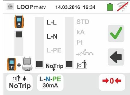
3. Move the left slide bar reference by selecting the RCD tripping time between the values: **6, 10, 30, 100, 300, 500, 650, 1000mA**
