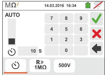
4. Touch the icon "R≥xxΩ" to set the minimum limit value of the insulation resistance on which the instrument makes the comparison with the measured value. The screen to the side appears on the display.
