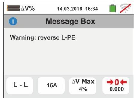
8. If the instrument detects a danger voltage on PE conductor, it does not carry out the test and displays a screen like the one to the side. This message can also appear in case of an insufficient pressure of the **GO/STOP** key
