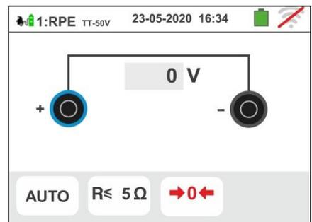
8. The value of the result is shown in the upper part of the screen while the partial values of the tests with inverted polarity of the test source in addition to the actual test currents are shown in the fields "R +" and "R-"
