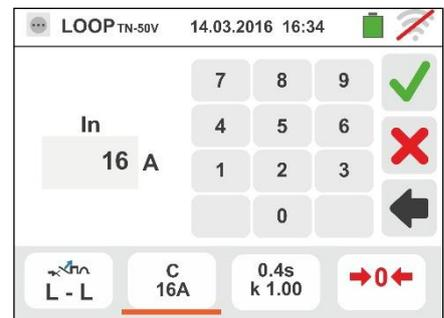
5. Move the slide bar reference by selecting the protection tripping time between the options: **0.1s**, **0.2s**, **0.4s**, **1s**, **5s**. Confirm the choice by going back to the initial measurement screen.
