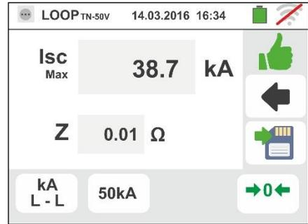
6. In case of test failure (measured Isc Max current > set threshold), the screen to the side is displayed by the instrument.
