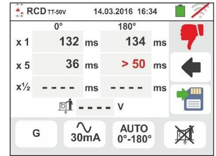
11 The test has a positive result if all tripping times of **molded case type STD** comply with what indicated in Table 6 (see § 13.4). The test has a negative result when one of the values is out of range. During this whole stage, do not disconnect the measuring leads of the instrument from the system on test.
