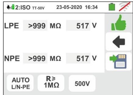
14 For three-phase EVSE systems, the measurement result of the **first L1PE test** is shown in the screen to the side. The values of the real test voltages are shown on the display
