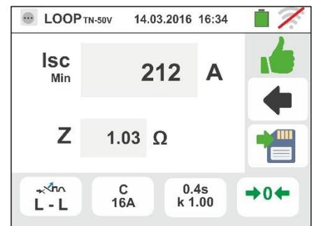
9. In case of negative result (minimum short-circuit current NOT interrupted by the protection device within the time indicated by the performed selections), the screen to the side is displayed by the instrument. Note the presence of the measurement result highlighted in red.
