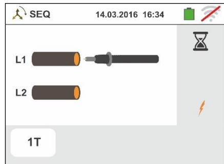
6. At the end of phase L1 acquisition, the instrument is in standby waiting for the signal on phase L2 and showing the symbol of "disconnected tip" as shown in the screen to the side.
