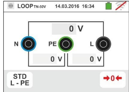
2. Touch the icon in order to select the test leads calibration or the icon to select the cable with Shuko plug calibration as shown in the following screen
