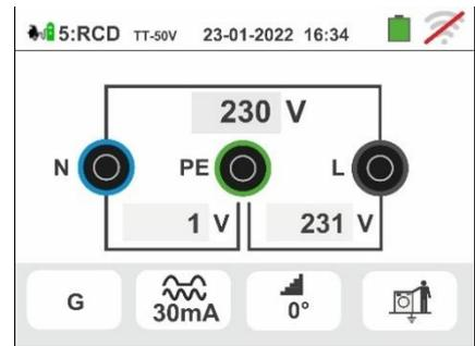
58 Move the third slide bar reference by selecting the desired rated current of the differential switch between the options: **6,10, 30, 100, 300, 500, 650mA**
