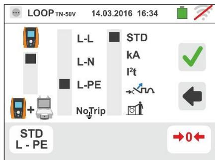
3. If possible, disconnect all loads connected downstream of the measuring point, as the impedance of these users could distort the test results.
