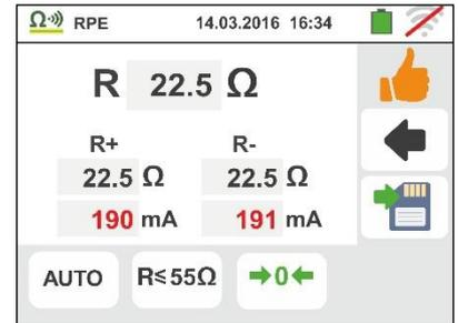
2. If in "→0←" mode the instrument detects a resistance higher than 5Ω at its terminals, it resets the offset value and displays a screen like the one to the side. The "→0←" icon is shown on the display to indicate the calibration reset value (i.e. performing the operation with open terminals).
