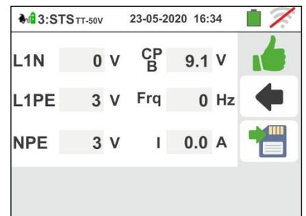
29 If the test fails, the screen like the one on the side is shown on the display. The incorrect value of the parameter is shown in red and the symbol indicates the non-ok result of the measurement.
