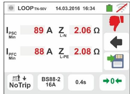
9. If the electrical Noise between N and PE conductors is so high that it could compromise the result accuracy, the symbol
