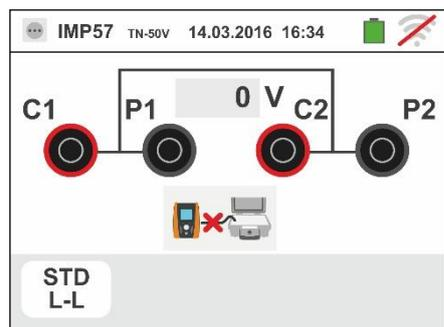
4. The symbol indicates the correct connection and recognition of the IMP57 by the instrument. Check the green STATUS LED lighting on the IMP57.
