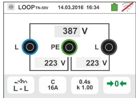
8. Press the **GO/STOP** key for few seconds or the **START** key on the remote lead. During this whole stage, do not disconnect the measuring leads of the instrument from the system under test.
