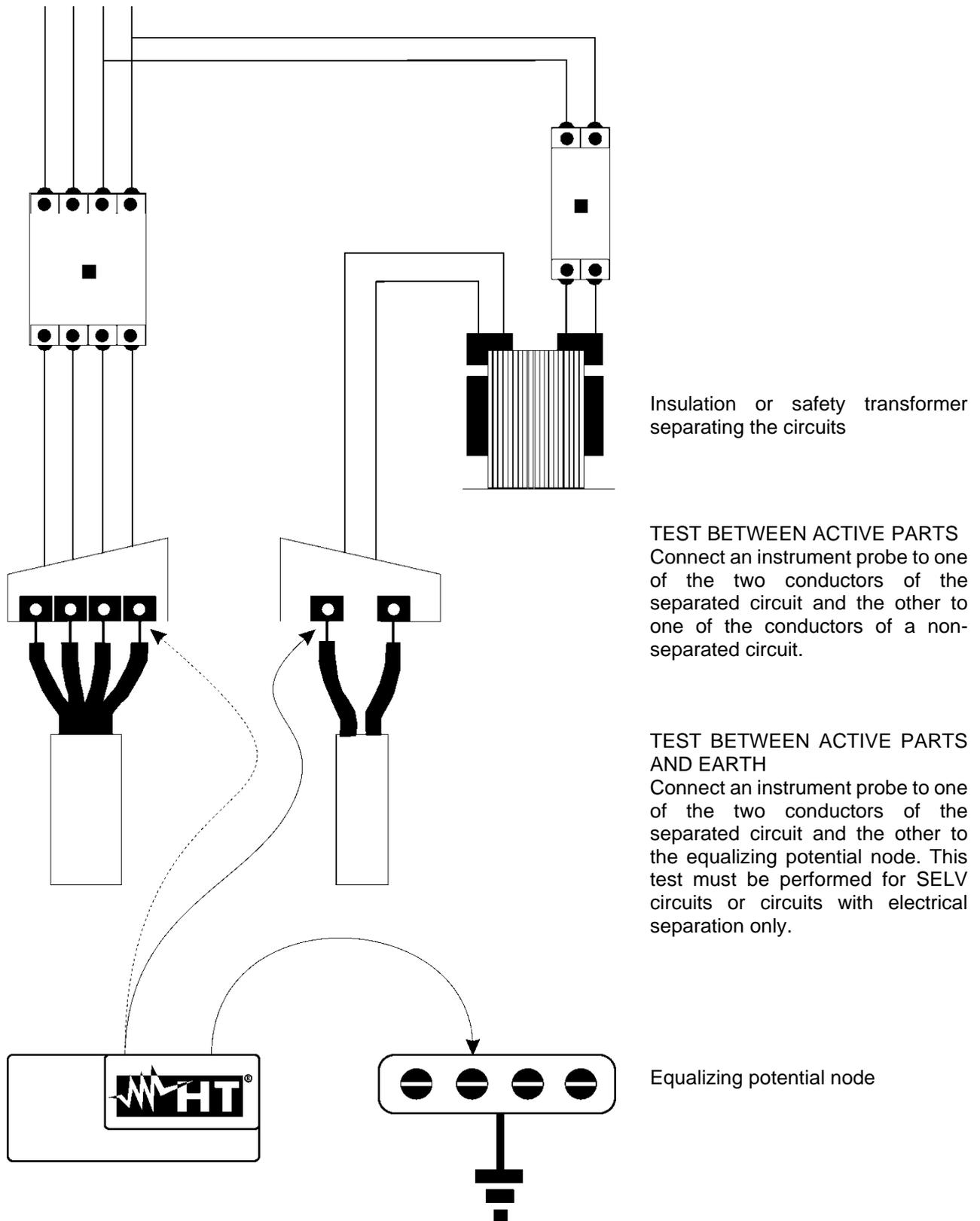
Fig. 45: Separation measurements between the circuits of a system
