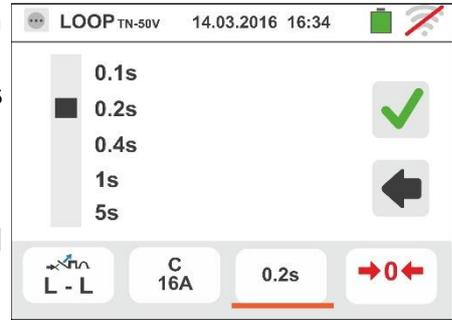
6. If possible, disconnect all loads connected downstream of the measured point, as the impedance of these users could distort the test results. Perform the preliminary calibration of the test leads as described in § 6.4.2 Connect the shuko plug, the alligator clips or the remote lead to the electrical mains according to Fig. 18, Fig. 19, Fig. 20 and Fig. 22 in the farthest possible point respect the protection on test
