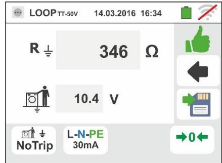
Press the **SAVE** button or touch the
