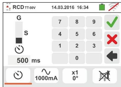
4. Move the left slide bar reference and select the type of RCD between the following options: **STD** (molded case RCD) and
