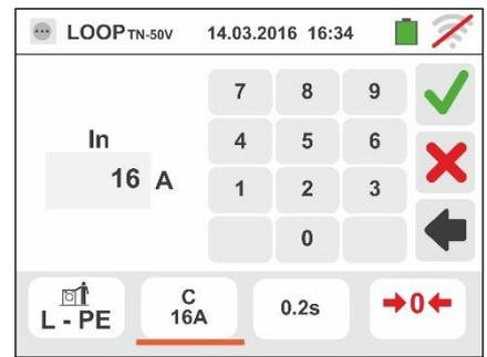
5. Move the slide bar reference by selecting the protection tripping time between the options: **0.1s, 0.2s, 0.4s, 1s, 5s** (all countries except AUS/NZ and UK), **0.4s, 5s** (Fuse protection for AUS/NZ and UK) and **0.4s** (MCB protection for AUS/NZ)
