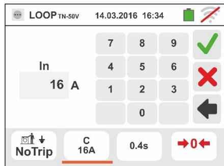
5. Move the slide bar reference by selecting the protection tripping time between the options: **0.1s**, **0.2s**, **0.4s**, **1s**, **5s** (all countries except AUS/NZ), **0.4s**, **5s** (Fuse protection for AUS/NZ) and **0.4s** (MCB protection for AUS/NZ)
