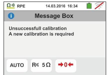
3. In case the instrument detects a calibration reset (performing the operation with open terminals), it gives out a long sound and displays a screen like the one to the side. The "→0←" icon is shown on the display to indicate the calibration reset value.
