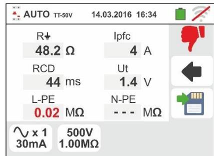
14 In case of **negative** result of the **MΩ N-PE**, the auto test is automatically blocked, the symbol is shown and the screen to the side is displayed. Note red value (lower than minimum set threshold) of the N-PE insulation resistance
