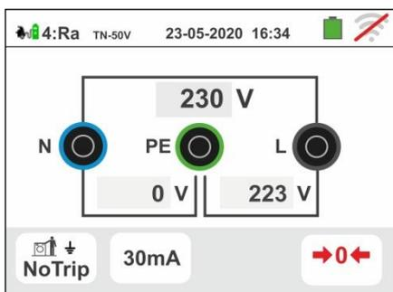
53 During this whole phase, do not disconnect the measuring terminals of the instrument from the system. In case of positive result ( $Z_{L-PE}$  or  $Z_{L-N}$  **LOWER or EQUAL to limit impedance relative to protection device within the specified time** – see § 13.7), the screen to the side is displayed by the instrument. Press again the **GO/STOP** key for a few seconds to repeat the test
