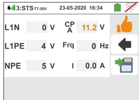
23 If the test fails, the screen like the one on the side is shown on the display. The incorrect value of the parameter is shown in red and the symbol
