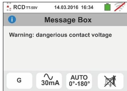
11 If the instrument detects a voltage  $V_{n-pe} > 50V$  (or the analogue  $V_{n-pe} > 25V$ ) it provides the warning screen shown to the side and blocks the test for safety reasons. Check the PE conductor and earth plant efficiency
