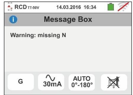
5. If the instrument detects the absence of the signal to terminal B3 (PE conductor), it provides the warning screen shown to the side and blocks the execution of the tests.
