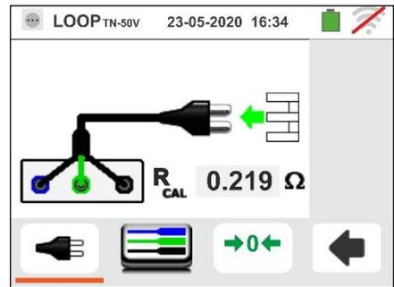
7. With open input terminals touch the
