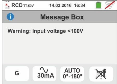
3. If the instrument detects the absence of the signal to terminal B1 (phase conductor), it provides the warning screen shown to the side and blocks the execution of the tests.
