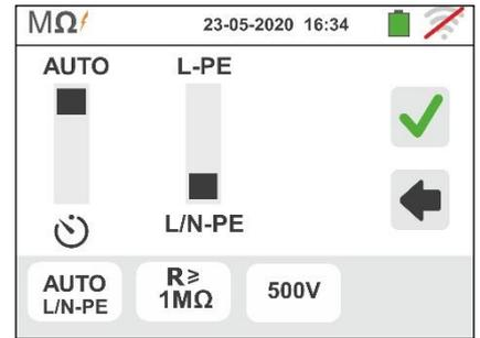
3. Touch the icon "R≥xxΩ" to set the minimum limit value of the insulation resistance on which the instrument makes the comparison with the measured value. The screen to the side appears on the display.
