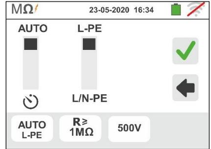
3. Touch the
