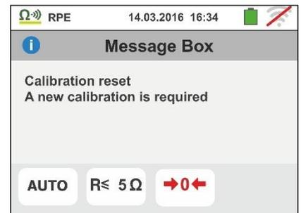
4. If the instrument detects a calibrated resistance higher than measured resistance (e.g. by using test cables different from the supplied ones) at its terminals, it gives out a long sound and displays a screen like the one to the side. Perform a calibration reset with open terminals and start a new calibration.
