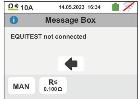
2. If you try to set a limit threshold value on the resistance measurement outside the permitted measurement range, the screen to the side is shown by the instrument. Set the limit value in the field: **0.003Ω ÷ 0.500Ω**
