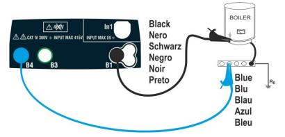
Fig. 10: Continuity test by means of single cables
