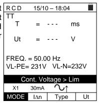
11. If the RCD does not trip within the maximum duration of the test, the instrument gives a long acoustic signal which signals the negative result of the test and then displays a screen similar to the one reported here to the side. Check that the set type of RCD matches the type of RCD being tested.
