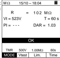
With a <u>measurement duration ≥ 600s</u>, the instrument MΩ shows the indication of the DAR parameter (Dielectric Absorbtion Ratio) and of the PI prameter (Polarisation Index) as shown in the screen to the side.
