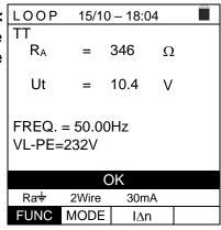
8. In case of **negative** result (**overall earth resistance** R<sub>A</sub> > LOOP (**Utlim/IΔn**), the "**NOT OK**" message and the screen to the side are displayed by the instrument. The screen contains the contact voltage value on the secondary display.
