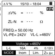
4. If the instrument detects a L-N or L-PE voltage higher than the maximum limit (265V), it does not carry out the test and displays a screen like the one to the side. Check the connection of measuring cables.
