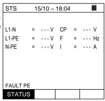
55. Press the **GO/STOP** key. The result of measurements is shown in the screen on the side. The instrument displays the message "**OK**" in case of a positive result of the tests (see Table 3)
