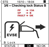
Use the keys ◀, ▶ to select the option "OK" in case of a positive result, and press the GO/STOP key to carry on with the test (see no. 35), or select the option "NO OK" and press the GO/STOP key to end the sequence of tests.
