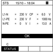
44. Press the **SAVE** key to partially save the test, and to carry on with the subsequent test (no. 53).
