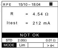
2. If the instrument detects a resistance higher than the full RPE scale, it emits a prolonged acoustic signal and displays a screen like the one to the side.
