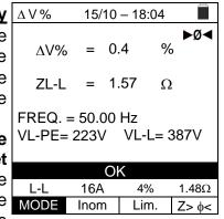
9. In case of negative result (maximum percentage value of calculated voltage drop according to § 12.11 > set limit value), the "NOT OK" outcome and the screen to the side are displayed by the instrument. The screen contains the value of the Z2 end-of-line impedance together with the Z1 (Offset) value.
