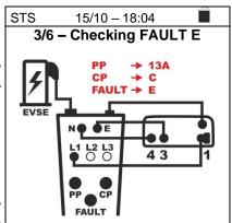
60. Press the **GO/STOP** key to start the test <u>on E status</u>. STS
