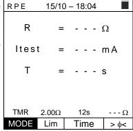
2. Press the **GO/STOP** key on the instrument or the **START** key on the remote switch probe. The instrument starts a series of continuous measurements for the entire duration set with a countdown, giving a short beep every 3 seconds and alternating the words "**Measuring...**" and "**Please wait...**".
