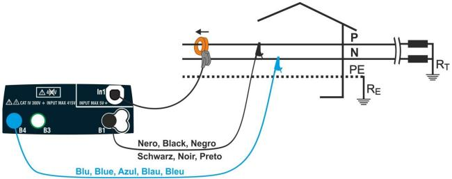
Fig. 42: Connection for measurements in a single-phase system
