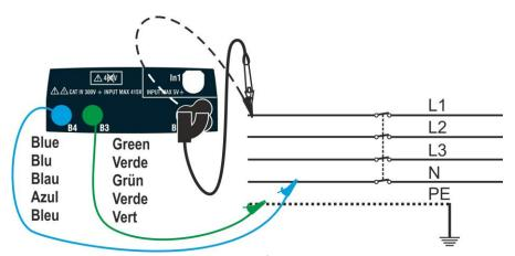
Fig. 9: Instrument connection by means of single cables and remote switch probe
