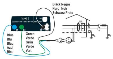
Fig. 19: Connection for single-phase L-N-PE system by means of mains plug
