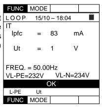
8. In case of **negative** result (contact voltage at the point >50V or >25V), the "**NOT OK**" message and the screen to the side are displayed by the instrument.
