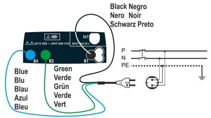
Fig. 8: Instrument connection through mains plug
