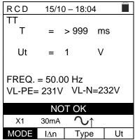
12. If the instrument detects, at the input terminals, too high an external impedance so that it cannot let the nominal current flow, it provides the warning screen shown to the side and blocks the test. Disconnect the possible loads downstream of the RCD before performing the test
