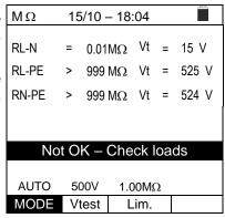
4. At the end of the test, if the value of the test voltage is lower than the nominal value, the instrument displays a screen like the one at the side.
