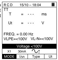
3. If the instrument detects a L-N or L-PE voltage higher than the maximum limit (265V), it does not carry out the test and displays a screen like the one to the side. Check the connection of measuring cables.
