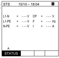
29. Press the **GO/STOP** key. The result of measurements is shown in the screen on the side. The instrument displays the message "**OK**" in case of a positive result of the tests (see Table 3)
