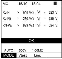
17. For split-phase EVSE systems, press the GO/STOP key on the instrument. The instrument starts the automatic test sequence of insulation resistance among L1-L2, L1-PE and L2-PE respectively, and displays the message "Measuring...". The instrument displays the message "OK" in case of a positive result of every test (value higher than the set minimum threshold).
