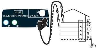
Fig. 36: Phase sequence check with remote switch probe
