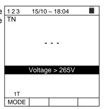
3. If, between the test start and the acquisition of the first voltage or between the acquisition of the first and second voltage, a time longer than approx. 10s has elapsed, the instrument displays a screen like the one to the side. It is necessary to repeat the test.
