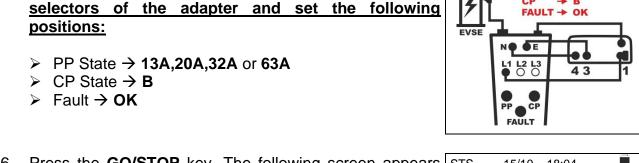
36. Press the **GO/STOP** key. The following screen appears on the display. Notice the presence of the status "**B**" corresponding to the position "STATUS"
