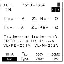
5. Press the **GO/STOP** key on the instrument or the **START** key on the remote switch probe. The instrument will start the automatic test sequence.
