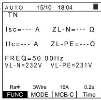
6. Press the **GO/STOP** key on the instrument, the **START** key on the remote switch probe or use the AutoStart feature (see § 5.1.5). The instrument starts the measurement and the "**Measuring**..." message is shown at display. During this whole stage, do not disconnect the measuring leads of the instrument from the system under test. The following screen appears on the instrument's display.
