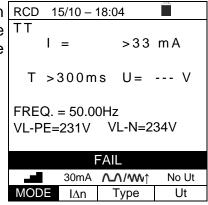
82. Press the **SAVE** key to partially save the test and to end the sequence of tests. The instrument shows the message contained in the following screen for a few seconds.
