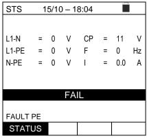
58. Press the **SAVE** key to partially save the test and to **end** the sequence of tests. The instrument shows the message contained in the following screen for a few seconds.
