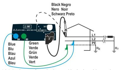
Fig. 34: L1-L2 3-wire test for splt-phase with single cables and remote probe
