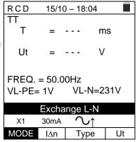
6. If the instrument detects that the phase and PE leads are inverted, it does not carry out the test and a screen similar to the one reported to the side is displayed. Check the connection of measuring cables.
