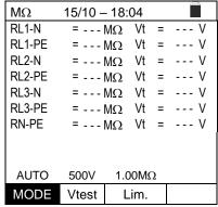
16. For single-phase EVSE systems, press the GO/STOP key on the instrument. The instrument starts the automatic test sequence of insulation resistance among L-N, L-PE and N-PE respectively, and displays the message "Measuring...". The instrument displays the message "OK" in case of a positive result of every test (value higher than the set minimum threshold).
