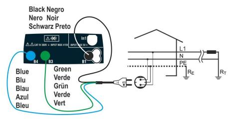
Fig. 25: L-N/L1-PE test for single-phase/split-phase systems with mains plug
