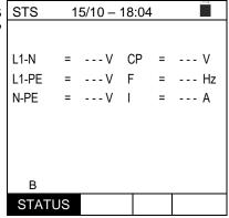
37. Press the **GO/STOP** key. The result of measurements is shown in the screen on the side. The instrument displays the message "**OK**" in case of a positive result of the tests (see Table 3).
