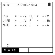
43. Press the **GO/STOP** key. The result of measurements is shown in the screen on the side. The instrument displays the message "**OK**" in case of a positive result of the tests (see Table 3).
