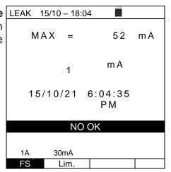
7. Press the **SAVE** key to store the test result in the instrument's memory (see § **7.1**) or the **ESC/MENU** key to exit the screen without saving and go back to the main menu
