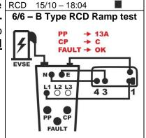
84. This test is carried out by the instrument by only considering standard STD (G) RCDs, of type B/B+ and in Ramp mode ( ) 0° (==/==+), no display of contact voltage Ut, rated current selectable among the following values: 6,10,30,100,300,500,650mA or type CCID === ↑) rated current selectable between 5,20mA. Please refer to § 6.6.4 for a description of the setting of the test parameters.
