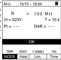
3. With a <u>measurement duration ≥ 60s</u>, the instrument MΩ shows the indication of the DAR parameter (Dielectric Absorbtion Ratio) as shown in the screen to the side.
