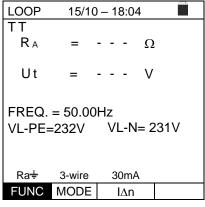
67. Press the **GO/STOP** key. The instrument will start measuring and the display will show the message "**Measuring**...". During this whole stage, do not disconnect the test leads of the instrument from the system being tested. The following screen appears on the display.
