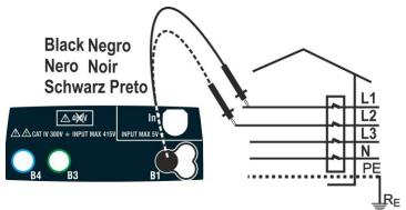
Fig. 35: Phase sequence check with test leads
