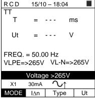
4. If the instrument detects a dangerous voltage on PE conductor, it provides the warning screen shown to the side and blocks the execution of the tests. Check the PE conductor and earth connection efficiency.
