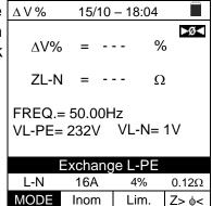
11. If the instrument detects a VL-PE, VL-N or VN-PE >5V during the test leads' calibration, it does not carry out the test and a screen similar to the one reported to the side is displayed. Check the connection of measuring cables.
