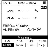
7. If the instrument detects the absence of the signal to terminal B4 (neutral conductor), it provides the warning screen shown to the side and blocks the execution of the tests.
