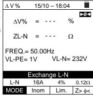
If the instrument detects that the phase and PE leads are inverted, it does not carry out the test and a screen similar to the one reported to the side is displayed. Check the connection of measuring cables.
