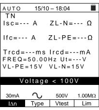
3. If the instrument detects that the phase and neutral leads are inverted, it does not carry out the test and a screen similar to the one reported to the side is displayed. Rotate the mains plug or check the connection of the measuring cables.
