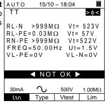
12. Press the **SAVE** key to store the test result in the instrument's memory (see § 7.1) or the **ESC/MENU** key to exit the screen without saving and go back to the main measuring screen.
