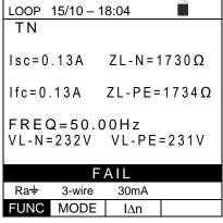
75. Press the **SAVE** key to partially save the test and to **end** the sequence of tests. The instrument shows the message contained in the following screen for a few seconds.
