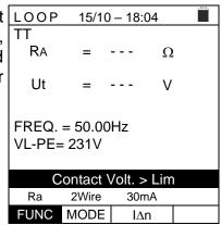
12. If the electrical noise between the N and PE conductors is so high that it compromises the uncertainty of the measurement result, the symbol is shown. It is recommended to disconnect all the utilities connected to the line and try the measurement again
