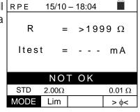
3. When using the >φ< mode, in case the instrument detects a calibration reset (performing the operation with open terminals), the instrument gives out a long sound and displays a screen like the one to the side.
