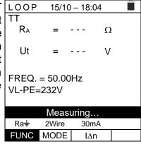
7. In case of **positive** result (**overall earth resistance** R<sub>A</sub> < LOOP (**Utlim/l**Δ**n**), the "**OK**" message and the screen to the side are displayed by the instrument. The screen contains the contact voltage value on the secondary display.
