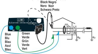
Fig. 22: Connection for L1-L2-PE split-phase system by means of single cables and remote switch probe
