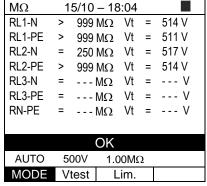
24. Press the **SAVE** key to partially save the test, and to carry on with the subsequent test (no. 26).
