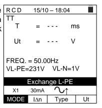
7. If the instrument detects the absence of the signal to terminal B3 (PE conductor), it provides the warning screen shown to the side and blocks the execution of the tests.
