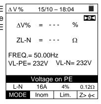
If the instrument detects the absence of the signal to terminal B1 (phase conductor), it provides the warning screen shown to the side and blocks the execution of the tests.
