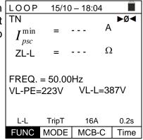
6. Press the **GO/STOP** key on the instrument, the **START** key on the remote switch probe or use the AutoStart feature (see § 5.1.5). The instrument starts the measurement and the "**Measuring...**" message is shown on the display. During this whole stage, do not disconnect the measuring leads of the instrument from the system under test. The following screen appears on the instrument's display.
