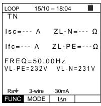
72. Press the **GO/STOP** key. The instrument will start measuring and the display will show the message "**Measuring**...".
