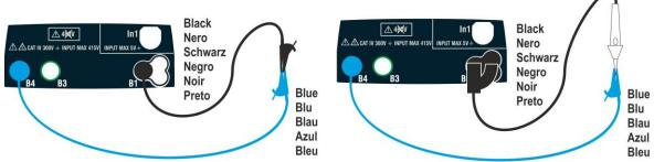
Fig. 12: Compensation of single cables and remote switch probe resistance
