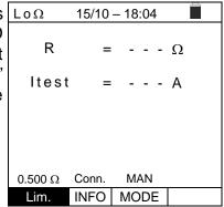
4. Use the ◀, ▶ keys to select the "INFO" item. The screen to the side is shown on the display indicating the information relevant to the EQUITEST accessory.
