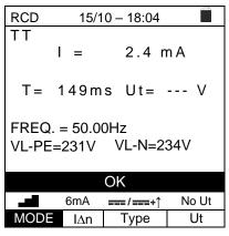
86. At the end of the test, if the tripping current is not within the values indicated in § 10.1, the instrument displays the message "FAIL" to indicate the negative outcome of the test and displays a screen like the one on the side.
