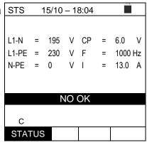
46. Press the **SAVE** key to partially save the test and to <u>end</u> <u>STS</u> <u>the sequence of tests.</u> The instrument shows the message contained in the following screen for a few seconds.
