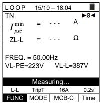
7. In case of **positive** result (minimum short-circuit current interrupted by the protection device within the time indicated by the performed selections), the "**OK**" message and the screen to the side are displayed by the instrument.  $I_{psc}^{min}$
