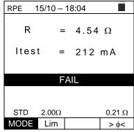
12. Press the **SAVE** key to partially save the test and to end the sequence of tests. The instrument shows the message contained in the following screen for a few seconds.
