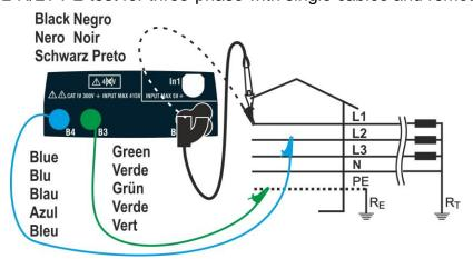
Fig. 28: L1-L2 measurement for three-phase systems
