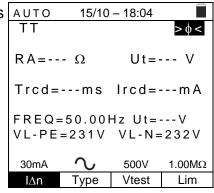
Press the GO/STOP key on the instrument or the START key on the remote switch 5. probe. The instrument will start the automatic test sequence.
