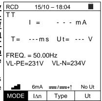
85. Press the **GO/STOP** key. The instrument will start measuring and the display will show the message "**Measuring**...". During this whole stage, do not disconnect the test leads of the instrument from the system being tested. The following screen appears on the display:
