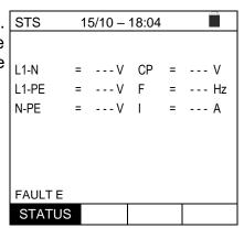
61. Press the **GO/STOP** key. The result of measurements is shown in the screen on the side. The instrument displays the message "**OK**" in case of a positive result of the tests (see Table 3)
