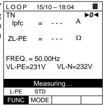
7. During this whole stage, do not disconnect the measuring RCD leads of the instrument from the system under test. The following screen appears on the instrument's display.
