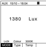
5. Press the **SAVE** key to store the test result in the instrument's memory (see § 7.1) or the **ESC/MENU** key to exit the screen without saving and go back to the main menu
