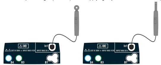
Fig. 39: Measurement of environmental parameters through external probes
