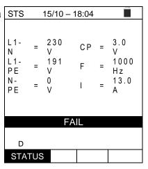
52. Press the **SAVE** key to partially save the test and to <u>end</u> <u>STS</u> the sequence of tests. The instrument shows the message contained in the following screen for a few seconds.
