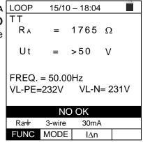
70. Press the **SAVE** key to partially save the test and to <u>end</u> <u>LOOP</u> the sequence of tests. The instrument shows the message contained in the following screen for a few seconds.
