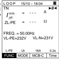
14. Press the **GO/STOP** key on the instrument, the **START** key on the remote switch probe or use the AutoStart feature (see § 5.1.5). The instrument starts the measurement and the "**Measuring...**" message is shown at display. During this whole stage, do not disconnect the measuring leads of the instrument from the system under test. The following screen appears on the instrument's display.
