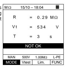
3. In AUTO mode, if the insulation measurement L-N is  $<50 k\Omega = 0.05 M\Omega$ , all the tests are completed or if the **STOP** key has been pressed, if RL-PE and RN-PE> Lim and Vt> Vnom, the instrument shows a screen like the one at the side. Disconnect the loads and resume the test.
