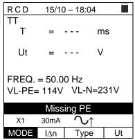
8. If the instrument detects the absence of the signal to terminal B4 (neutral conductor), it provides the warning screen shown to the side and blocks the execution of the tests.
