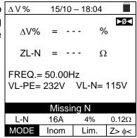
8. If the instrument detects the absence of the signal to terminal B3 (PE conductor), it provides the warning screen shown to the side and blocks the execution of the tests.  $\Delta V\%$
