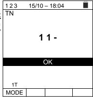
9. Press the **SAVE** key to store the test result in the instrument's memory (see § 7.1) or the **ESC/MENU** key to exit the screen without saving and go back to the main measuring screen.
