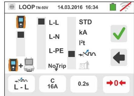
Mover a barra deslizante central seleccionando as opções “L-L”, “L-N” ou “L-PE”.
